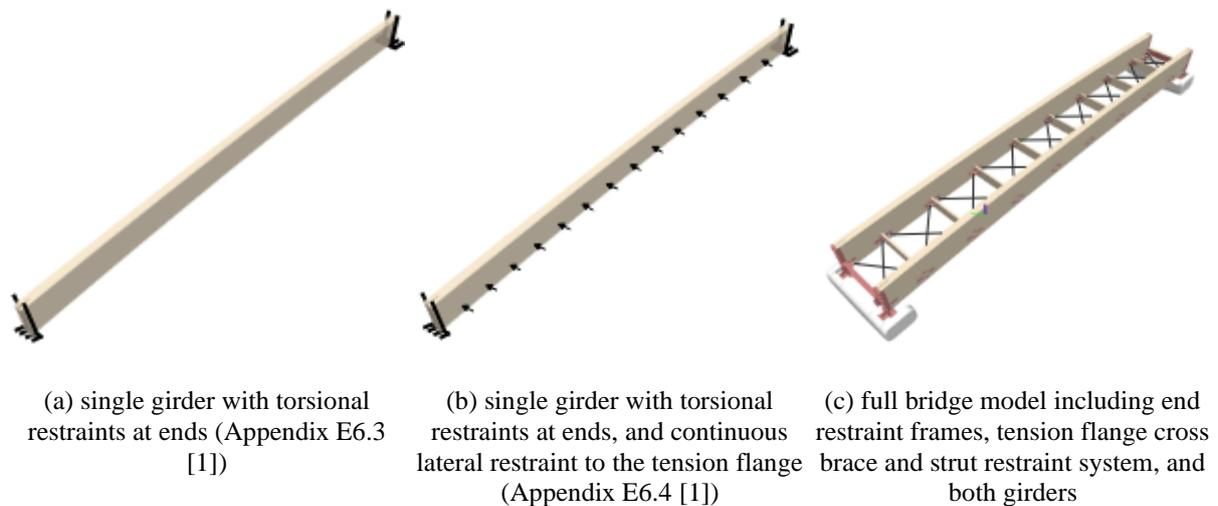
Figure 5. Visual representation of 3D ETABS models developed to verify analytical solutions
