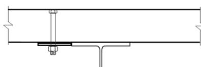
Figure 7 Sketch of Tab welded to flange, bolted to EPP
