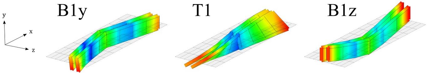
Figure 9. Experimental mode shapes for the finished arch section at stage 4 (MC3). The horizontal grid is in the xz-plane.
