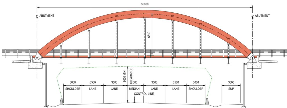
**Figure 1 Concept general arrangement long section.**
