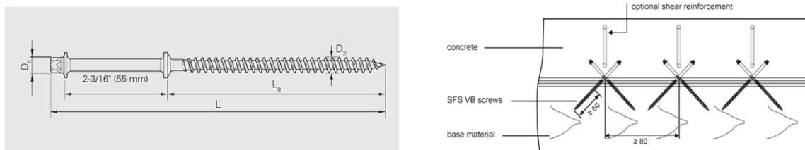
**Figure 4: Example of the proprietary fastener shear stud. SFS VB screws [10]**
