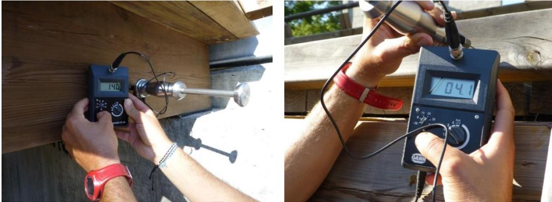
Figures 21 and 22. Big differences in the moisture content of the timber elements.
