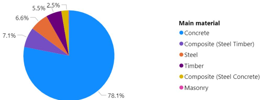
Figure 1. Summary of AT Bridges Constructed with Various Materials
