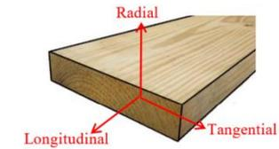
Figure 12. Principal axes of wood
