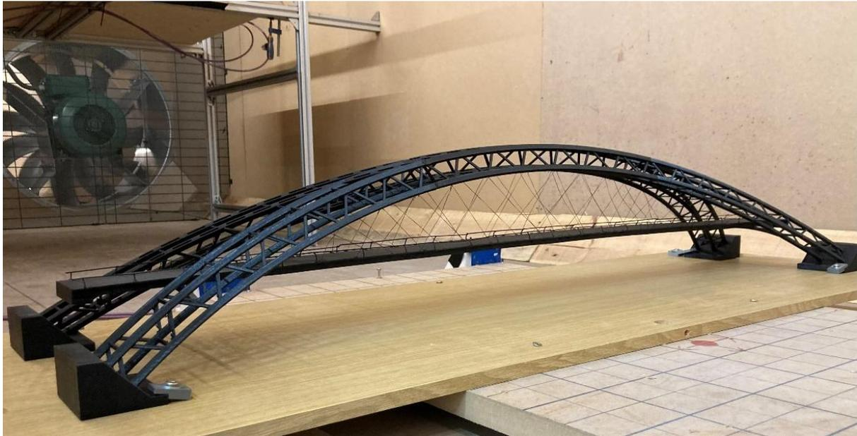
Figure 14 – Scaled model of the bridge
