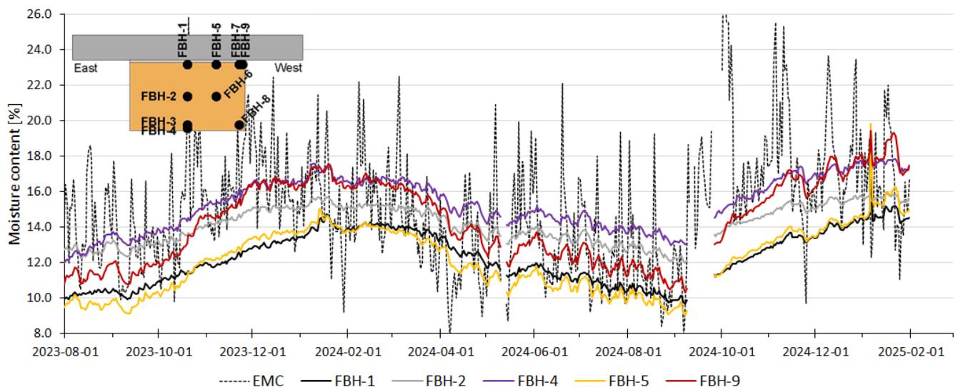
Figure 7. Daily mean values of equilibrium moisture content (EMC) and timber moisture content at five positions in measurement plane B (not sealed end grain)
