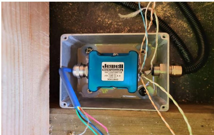
Figure 8: High-precision inclinometer for measuring the subsidence in the middle of the bridge
