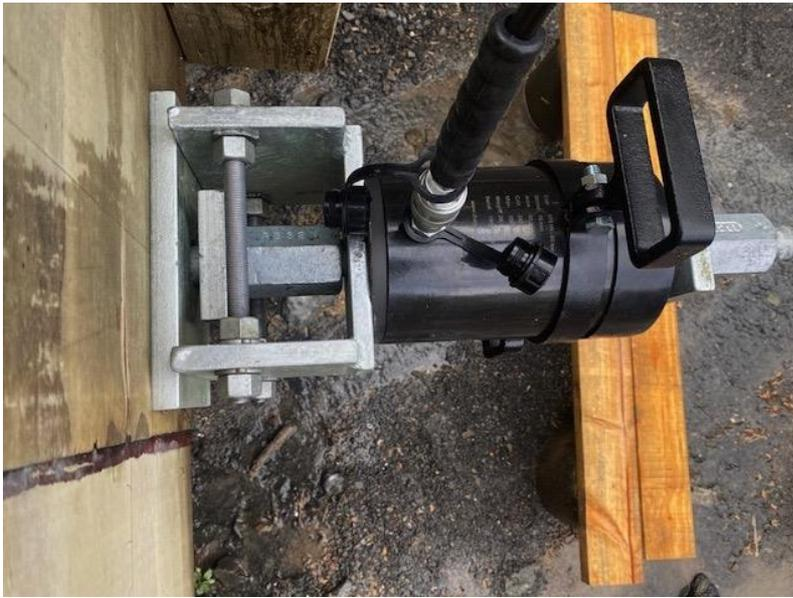
Photo 4: Hydraulic jack and stressing bridge used to calibrate the design tension in the pre-stressing bars stressed by applying torque.
