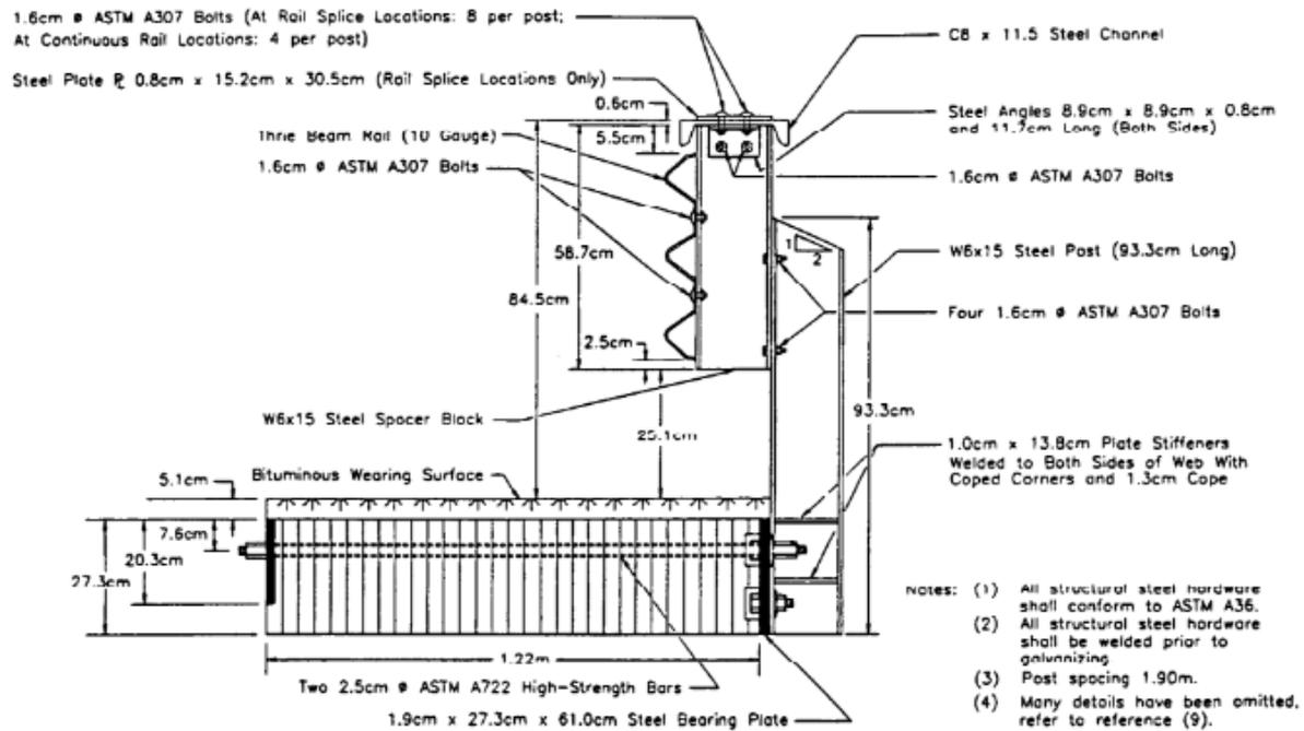
Figure 4 Example T1-4 barrier detail reproduced from Transport Research board [2]
