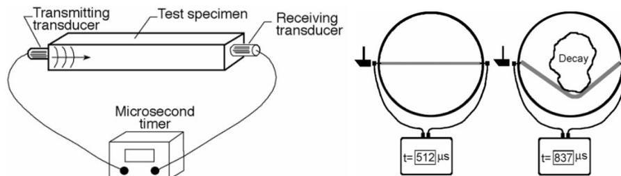
Figure 5. Stress wave timing (a) Test set-up [22]. (b) Reading comparison showing internal decay [23]
