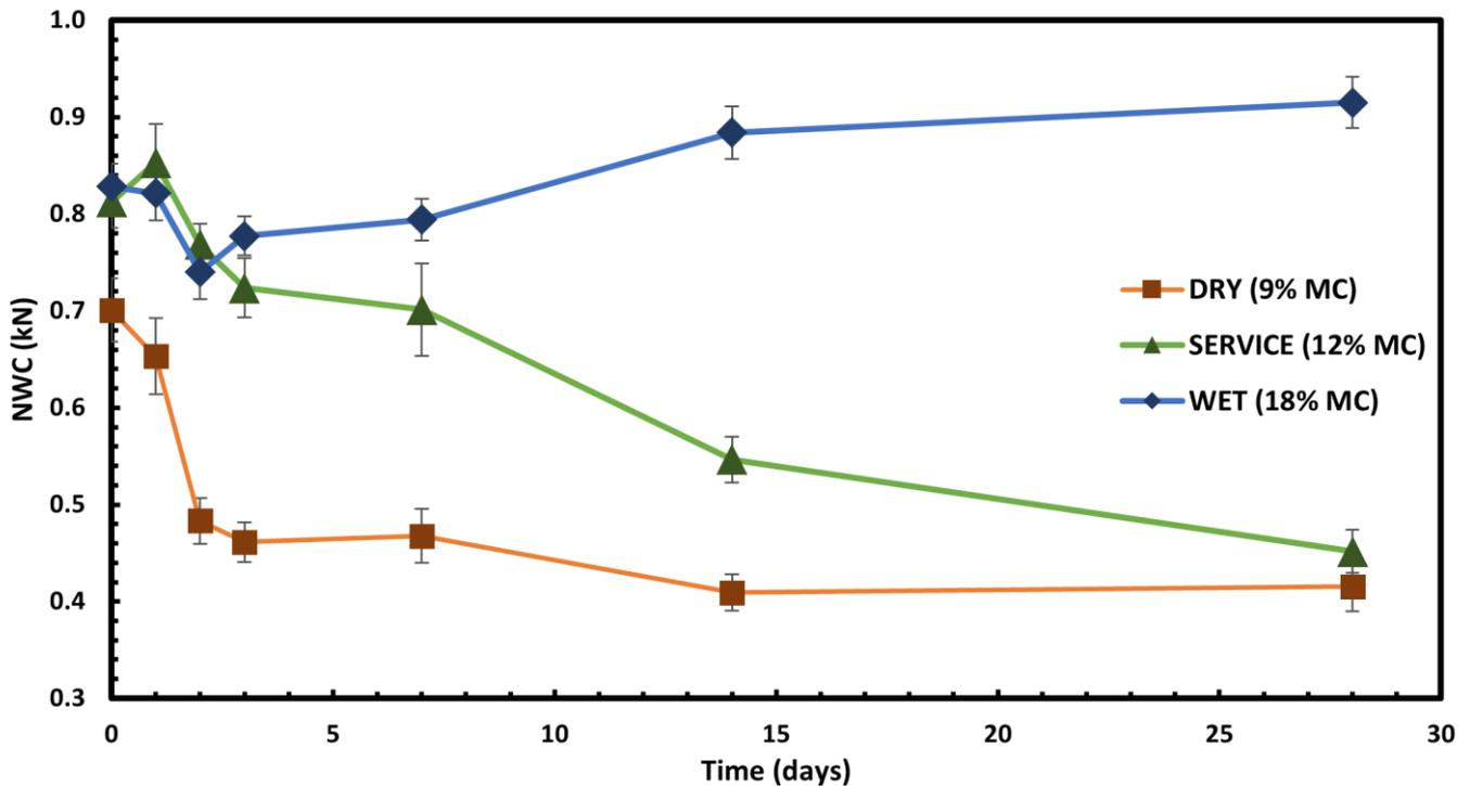
Figure 5. Average NWC changes from 0 to 28 days in DRY, SERVICE or WET. Error bars indicate standard errors.
