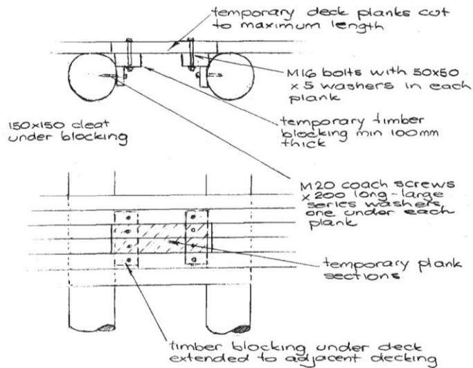
Figure 4. Indicative temporary deck repair for Drayton Rail Overbridge (Source: TMR TBMM [2])
