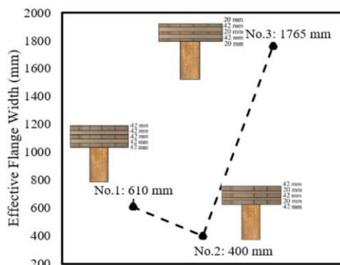
Figure 13. Effect of the layer's configuration change on the effective flange width for Configurations 1, 2, 3.
