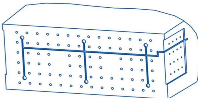
Figure 3: Position of resistive moisture sensor in principal
