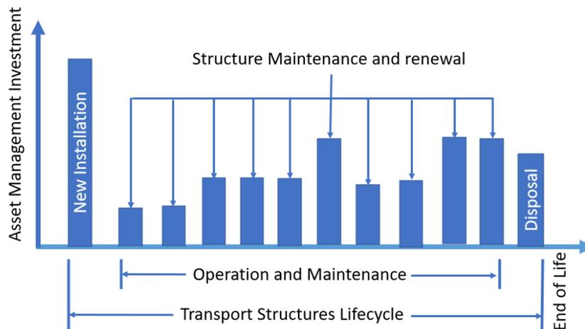
Figure 5. Lifecycle of a bridge
