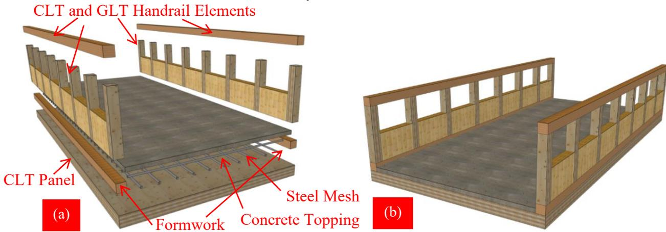
Figure 4. Prefabricated CLT bridge; a) before assembly, b) after assembly.
