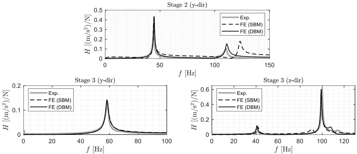
Figure 10. FRFs at stages 2-3 from hammer excitation and acceleration in the y- and z-direction.
