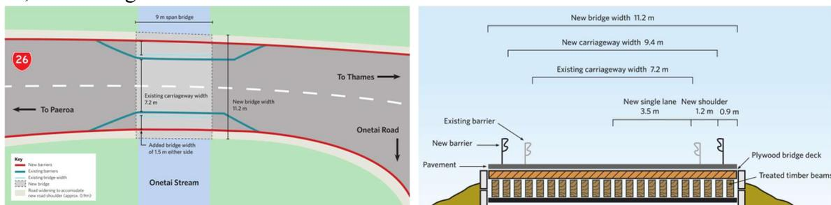
Figure 4. Plan view of the proposed bridge (left) and the proposed bridge cross-section (right) [17].
