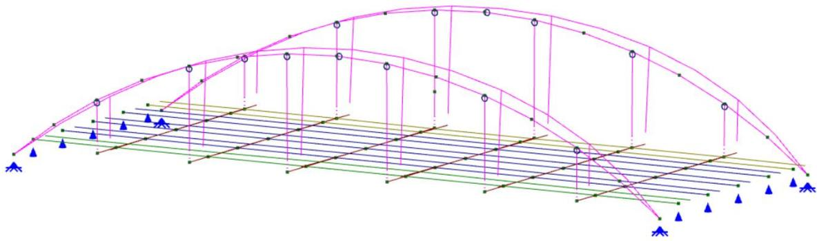
**Figure 3 Arch buckling shape.**
