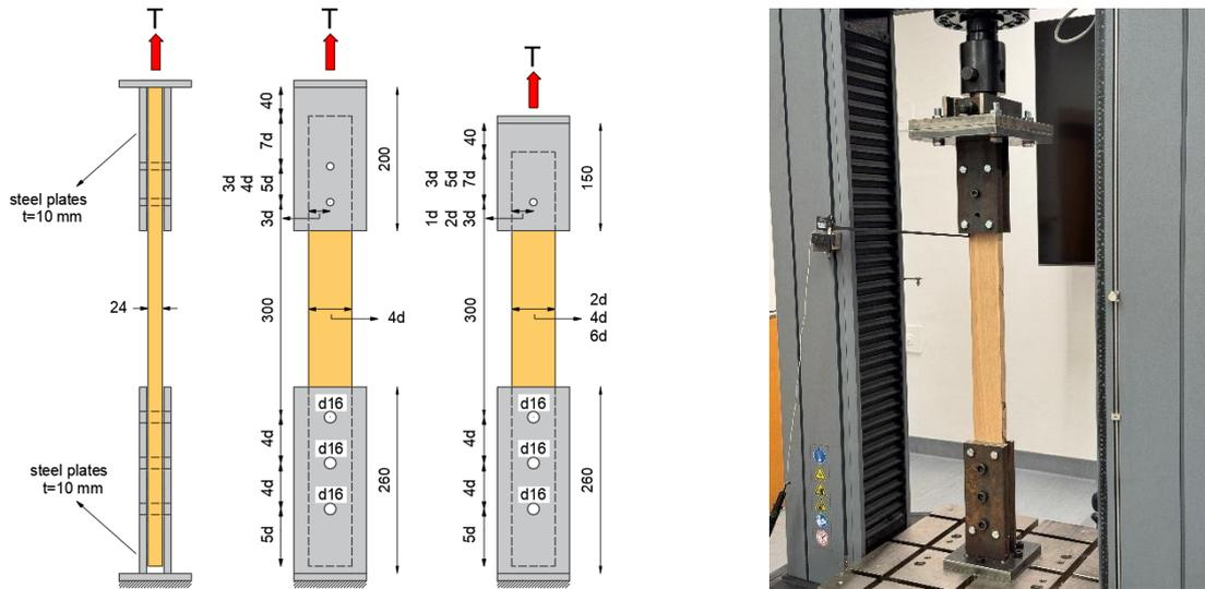
Figure 3. Details of the connection test setup (units: mm)
