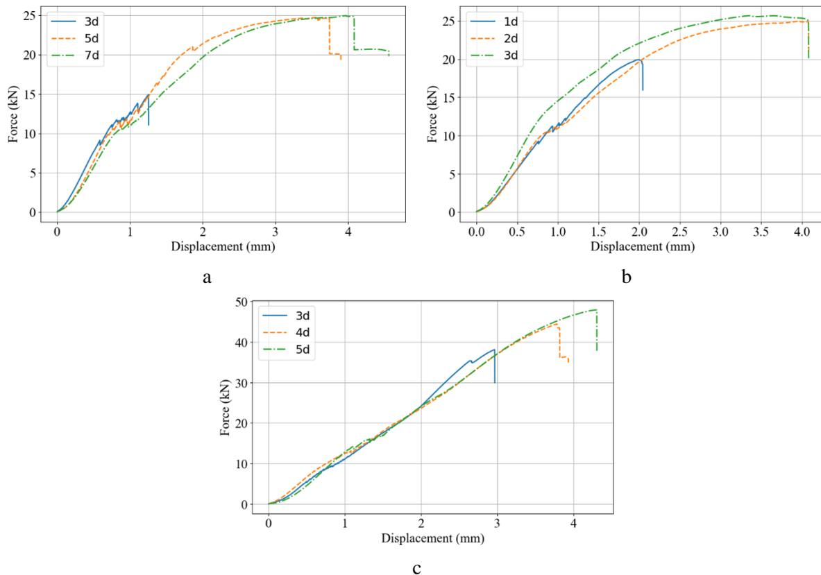
Figure 6. Average force-displacement curves showing the effect of (a) end distance (3d, 5d, 7d), (b) edge distance (1d, 2d, 3d), and (c) dowel spacing (3d, 4d, 5d) on connection performance.
