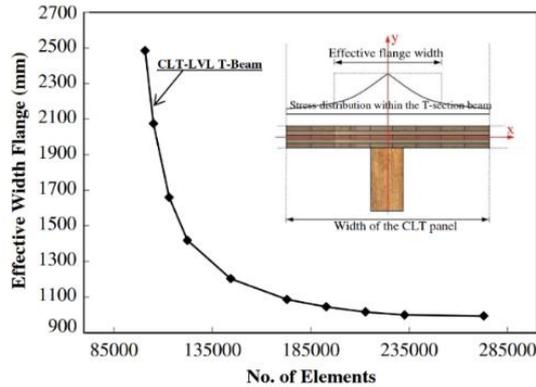
Figure 14. Convergence study result of EWF of CLT composite beam versus number of mesh elements.
