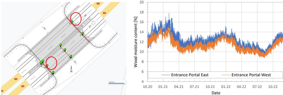
Figure 10. Measuring plan of Rynetel – wildlife overpass (left), measuring result of moisture content at the entrance portals
