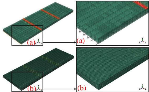
Figure 10. Typical boundary conditions and finite element mesh. (a) FE model boundary conditions (Load and support), (b) Finite element mesh.
