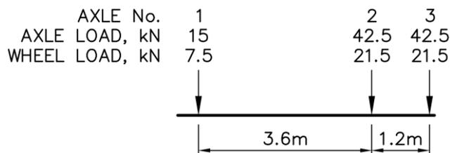
Figure 11. 10-tonne design live load vehicle
