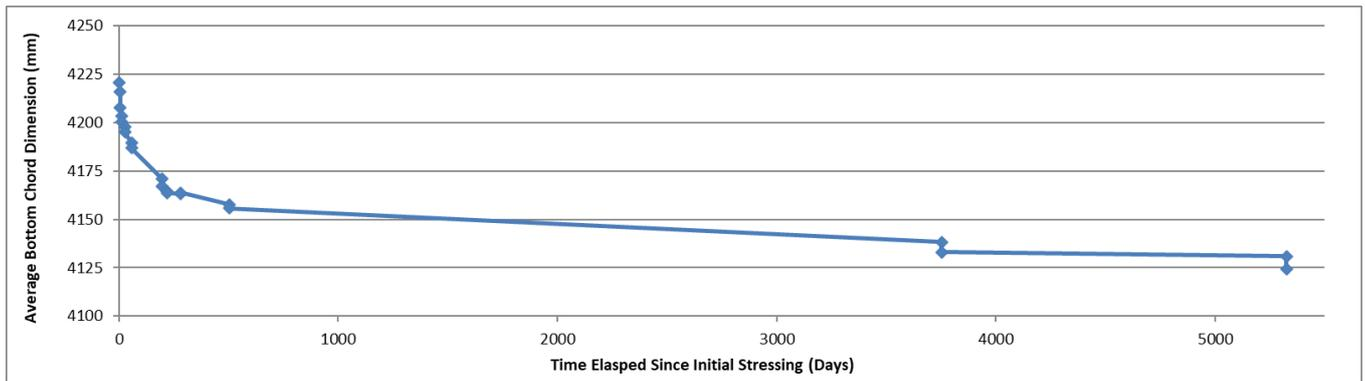
Figure 7. Narrowing of bottom chord of the bridge deck over 15 years.
