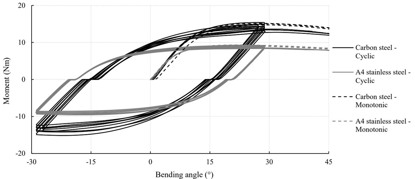
Figure 8. Cyclic bending test of partially threaded screws with nominal diameter  $d= 6.0$  mm and different material, carried out by assuming a low cycle ductility class S3.
