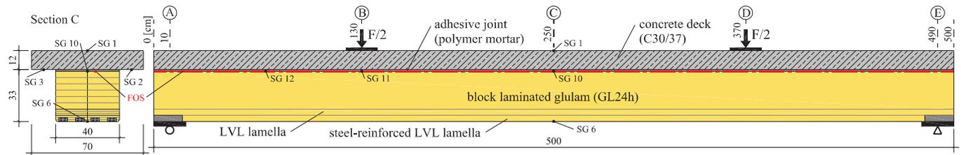
Figure 1: Specimen dimensions of the ATCC beams HBV-11 and HBV-12 used for the four-point bending tests with fibre-optical strain measurement along the adhesive joint
