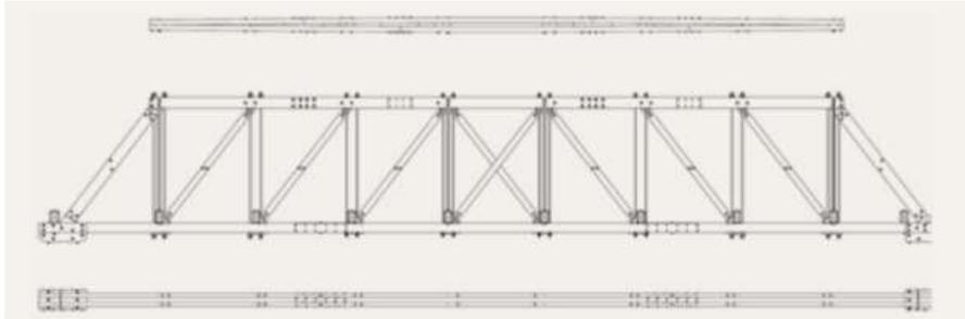
Figure 1. Typical Allan truss design [2]
