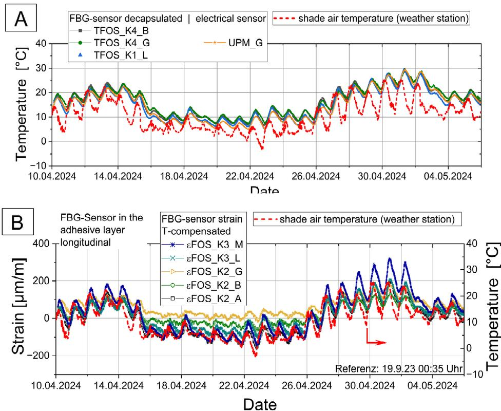
Figure 6: FBG-sensor data from the ATCC superstructure segment for approx. one month in outdoor climate Weimar, Germany: A) Temperature; B) Strain data compared with shade air temperature from weather station
