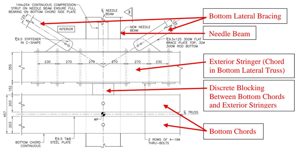
Figure 15. Excerpt of bottom lateral truss details.
