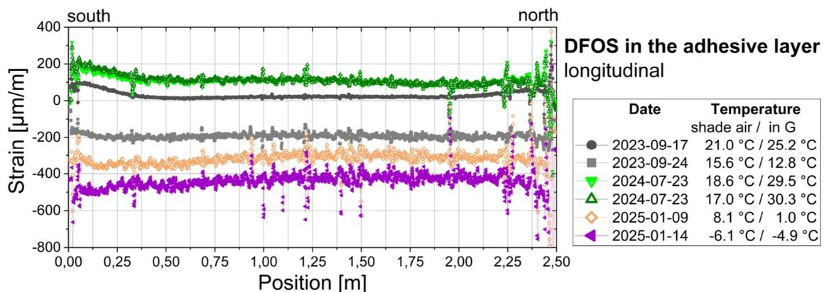
Figure 7: DFOS-data with spatial resolution of 1.3 mm from measuring campaigns of the ATCC superstructure segment in outdoor climate Weimar, Germany
