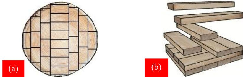
Figure 1. CLT production process; (a) Sawing log, (b) Arranging boards and final CLT product.
