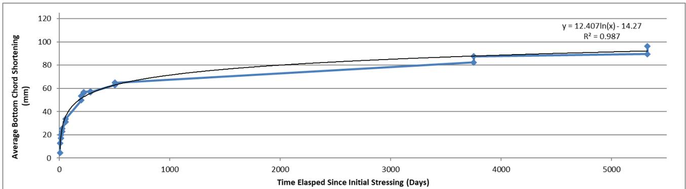
Figure 8. Compressive distortion of the bottom chord over 15 years, with creep curve.
