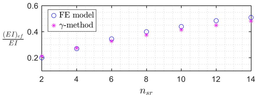
Figure 11. Reduction factor  $\frac{(EI)_{ef}}{EI}$  based on number of steel rod connections ( $n_{sr}$ ) along the MC2.
