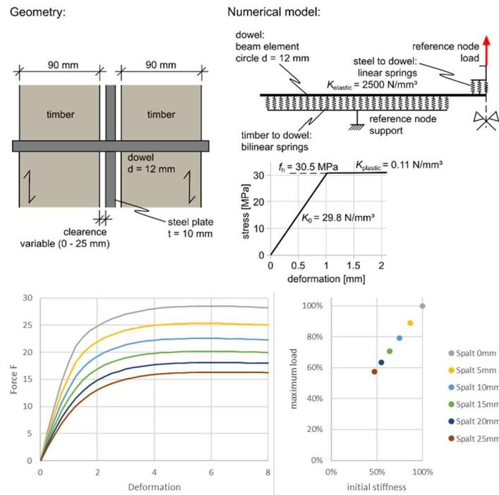
Figure 10. Numerical model setup of the knife plate connection with a single dowel embedded in timber with increasing gaps, load-deformation graphs (left) and slip modules (right)
