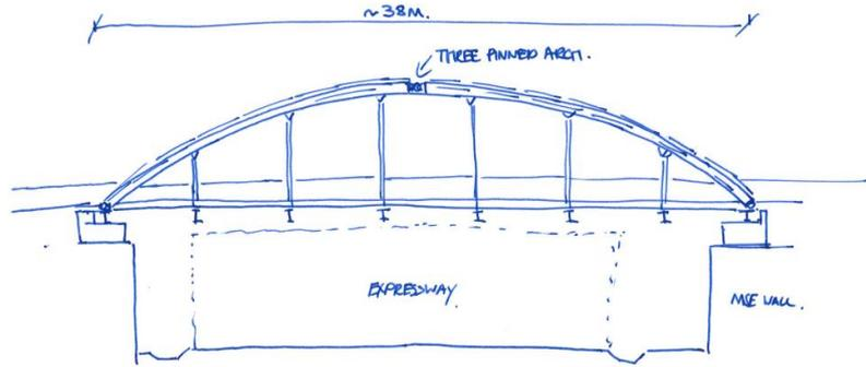
Figure 2. Sketch of engineered timber bridge considered in carbon calculations
