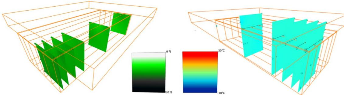
Figure 10. Visualisation of the measurement data in a digital model; left: Timber moisture distribution; right: Material temperature distribution
