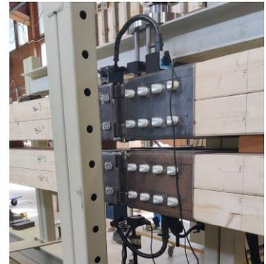
Figure 5. Experimental setup and measurement of the rotations at stage 4.
