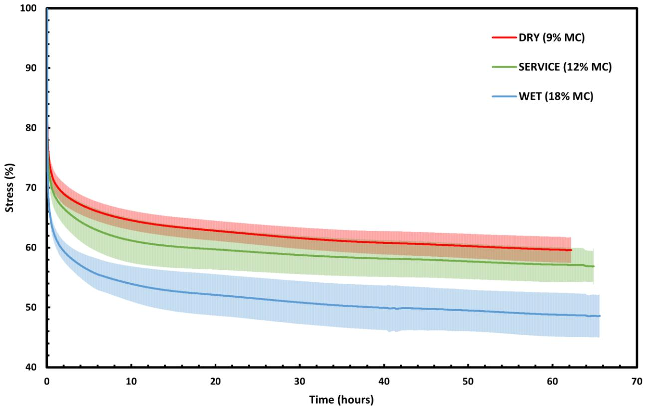
Figure 6. Average stress retention curves from 0 to 62 hours in DRY, SERVICE and WET. Shaded areas indicate standard deviation.
