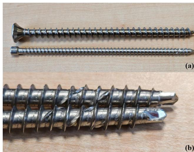
Figure 3. Fully threaded screws made of A4 austenitic stainless steel: (a) complete length of the screws with needle tip type, (b) close-up on the drill tip type variant of these screws.
