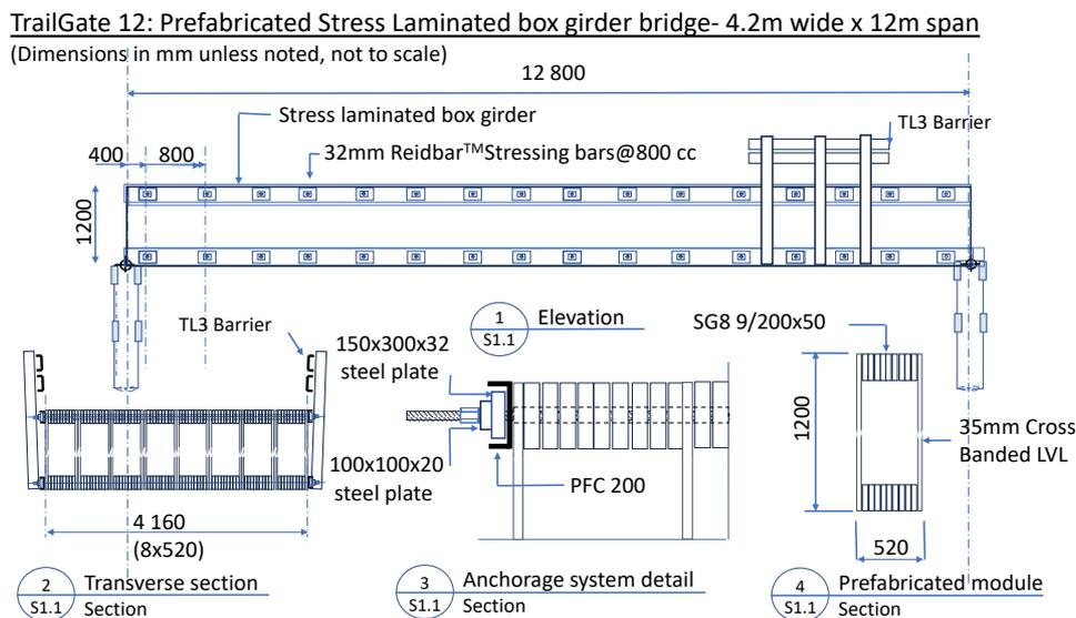
Figure 1: Concept design sketch of TrailGate 12: Stress laminated box girder bridge (12m span)
