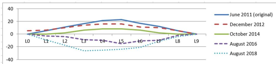
Figure 8. Truss deflection survey data along the truss span at each node
