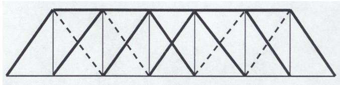
Figure 7. The General Form of a Howe Truss
