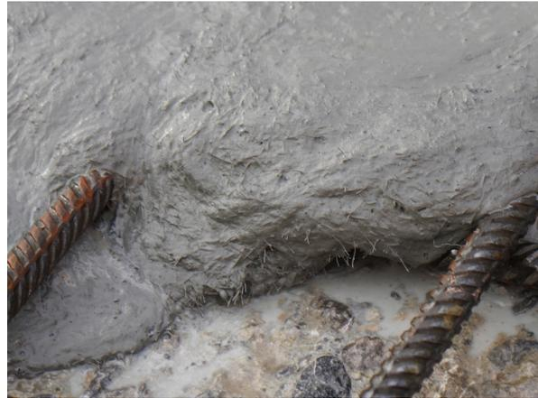
Figure 6: UHPFRC on a roughened concrete surface
