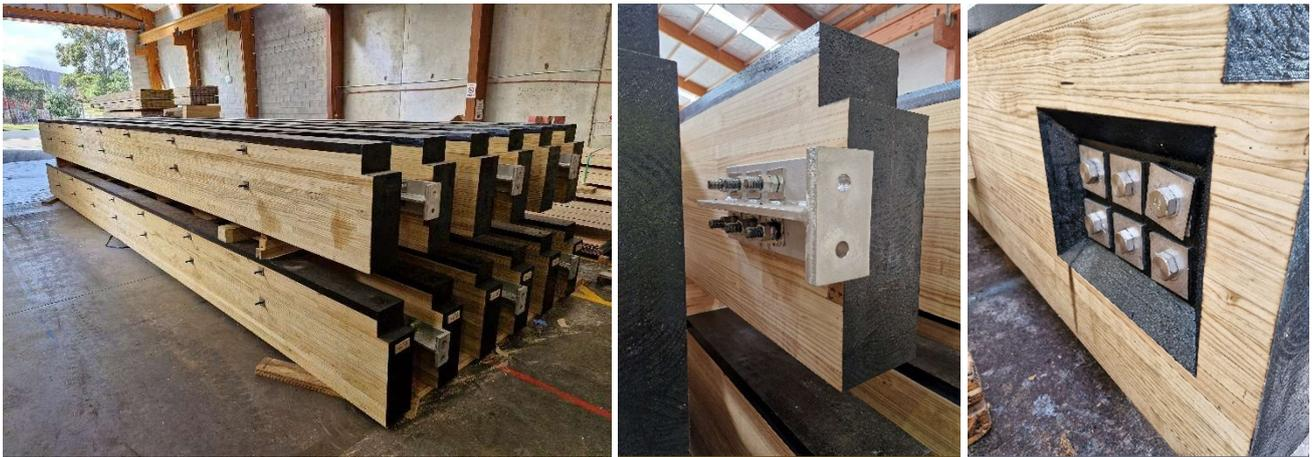
Figure 7. Timber girder modules (left), abutment bracket (middle), and bracket notch (right) at RSTL Factory, Auckland.
