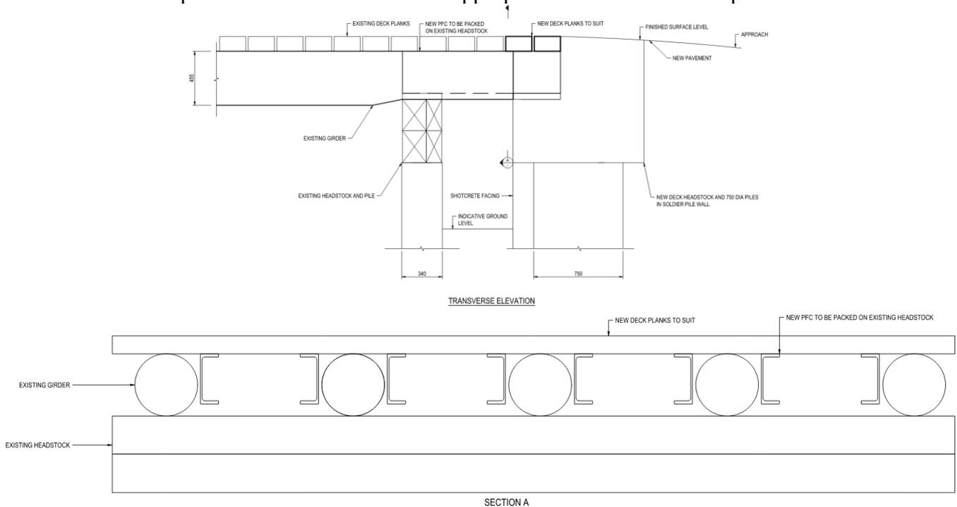
Figure 9. Bank end repair concept design at Hopes Road Rail Overbridge.
