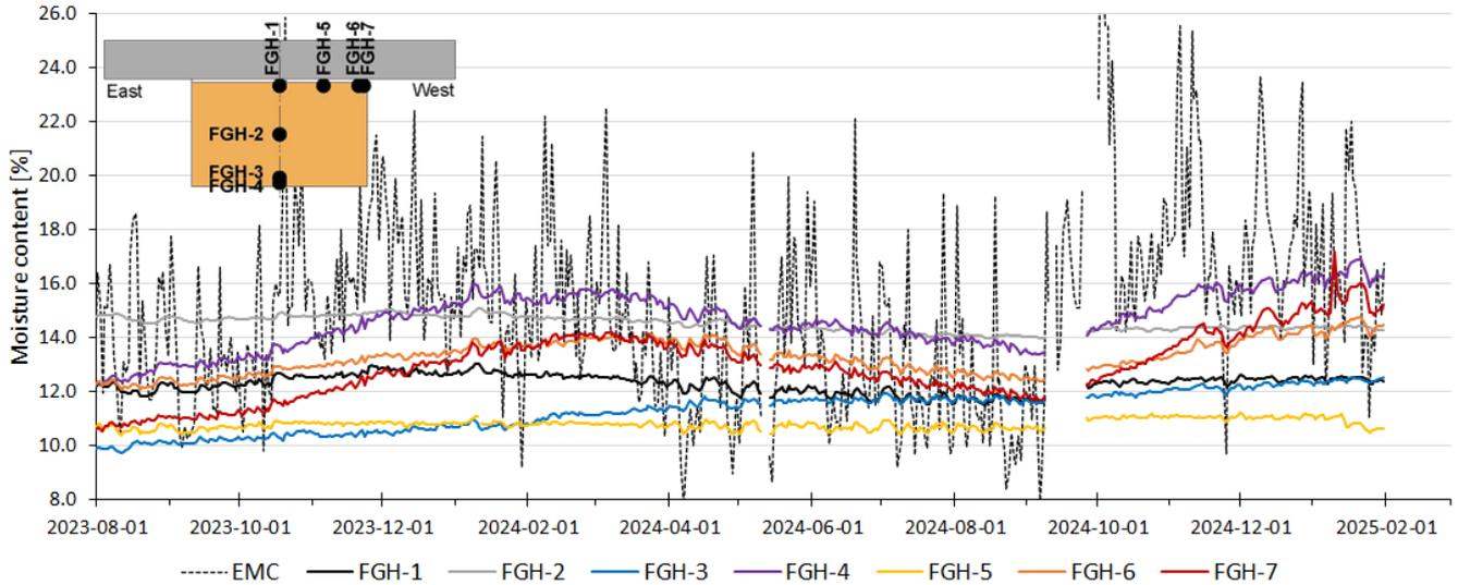
Figure 4. Daily mean values of equilibrium moisture content (EMC) and timber moisture content at several positions in measurement plane G (middle of the superstructure segment)
