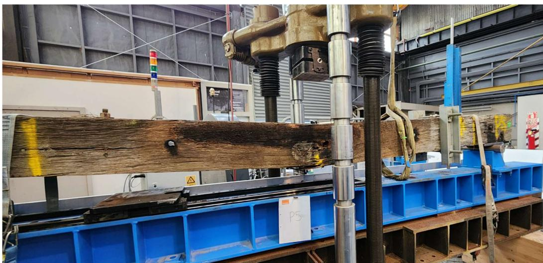
Figure 7: Test setup configuration for initial pile cap testing.
