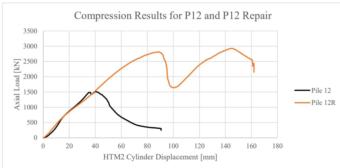
Figure 10: Comparison of pile performance before and after implementation of a split cylinder repair.
