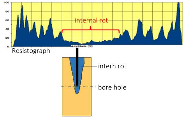
Figure 3. Klimm-Bridge: Joint with knife plates: Measurement of the moisture content (left) and drilling resistance at the bottom of the slotted-in steel plates (right)
