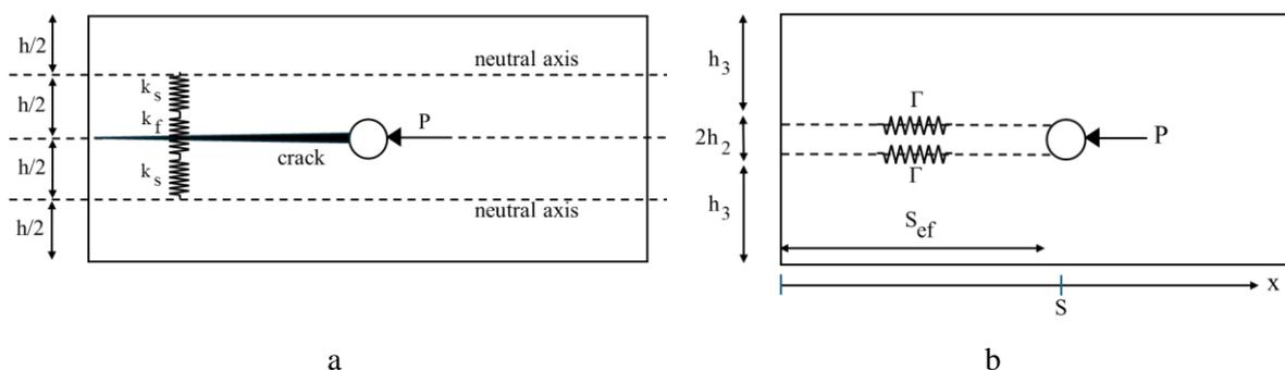
Figure 2. (a) Failure mode I: Splitting of the single-bolt connection loaded parallel to the grain. (b) Failure mode II: Row shear parallel in a single-bolt connection loaded parallel to the grain [11].
