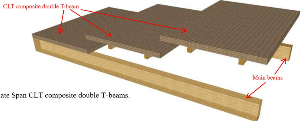
Figure 17. Intermediate Span CLT composite double T-beams.
