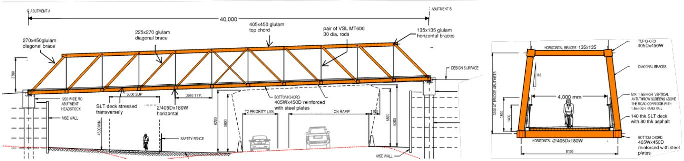
Figure 1 Initial concept design – elevation and cross section
