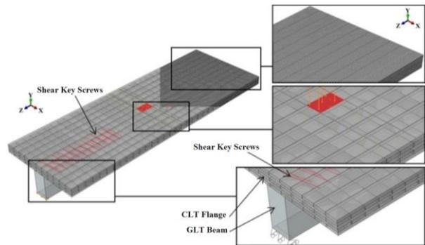
Figure 11. General arrangement of the numerical model to show boundary conditions and mesh.
