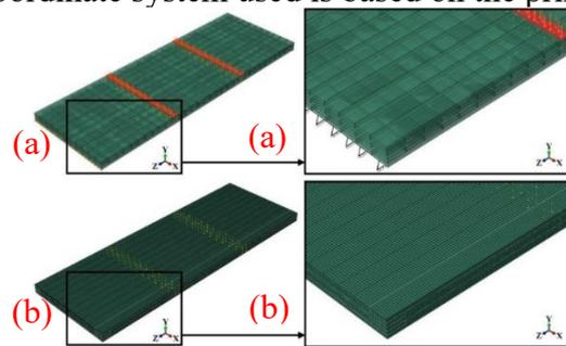
Figure 10. Typical boundary conditions and finite element mesh used in this study. (a) FE model boundary conditions (Load and support), (b) Finite element mesh.
