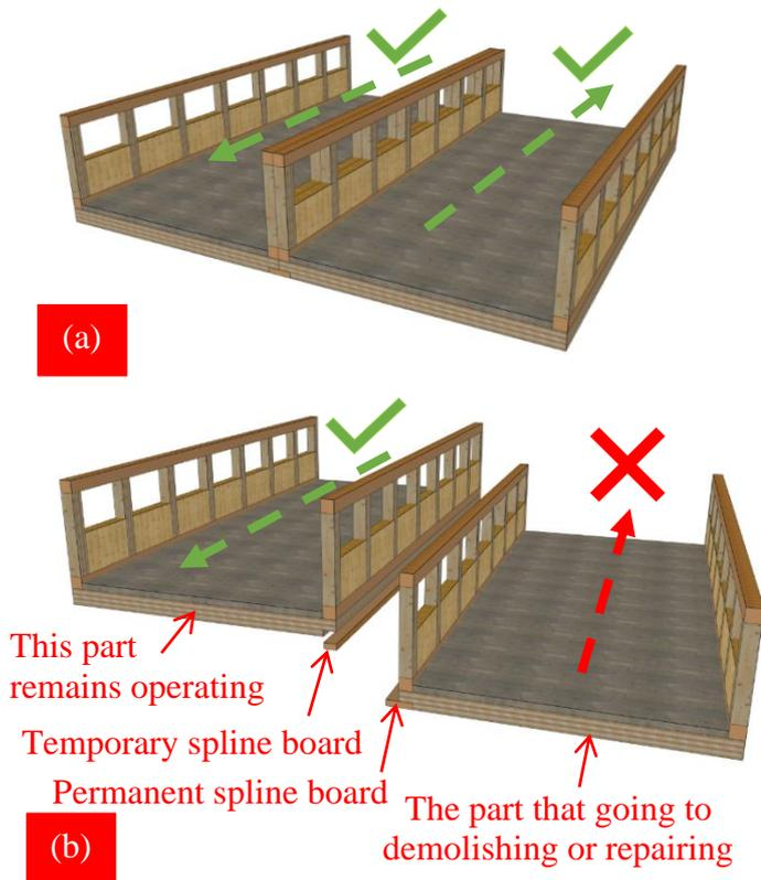
Figure 5. CLT bridge can remain semi-operational during the replacement of the old or damaged part of the bridge. a) fully operational, b) partially disassembled, and semi-operational.
