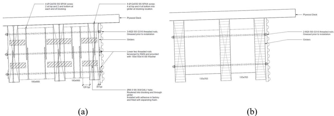
Figure 7: (a) Initial 'rigid' blocking detail, (b) Revised 'pinned' blocking detail.
