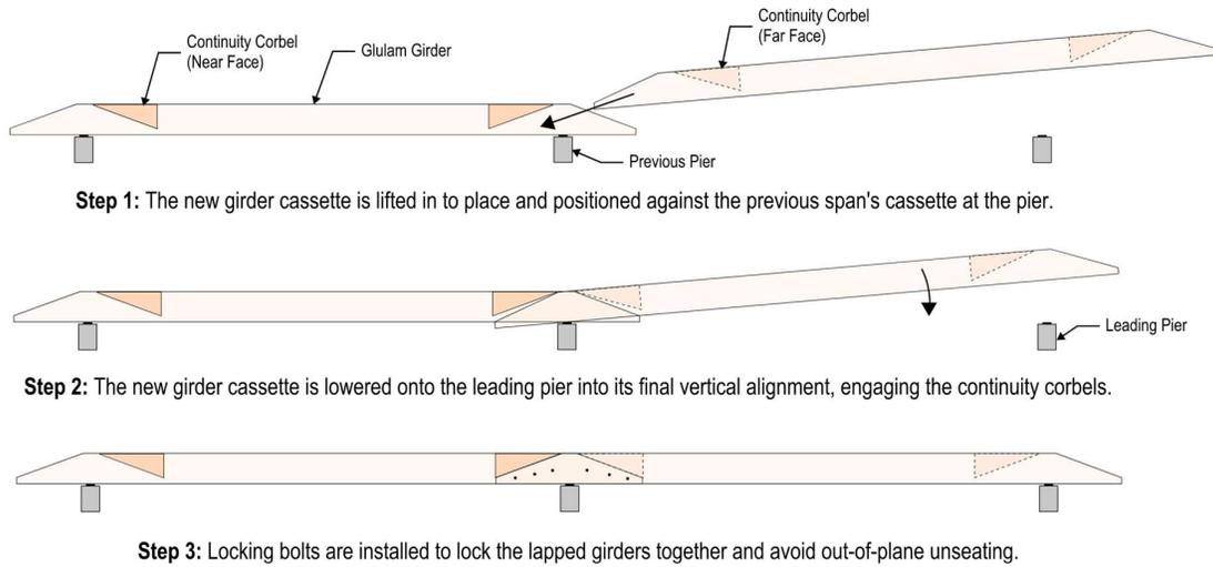
**Figure 4: Intended construction sequence for girder installation.**
