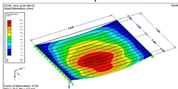
Figure 5. Dlubal RFEM for Onetai Stream Bridge showing calculated deflection under HN loading.
