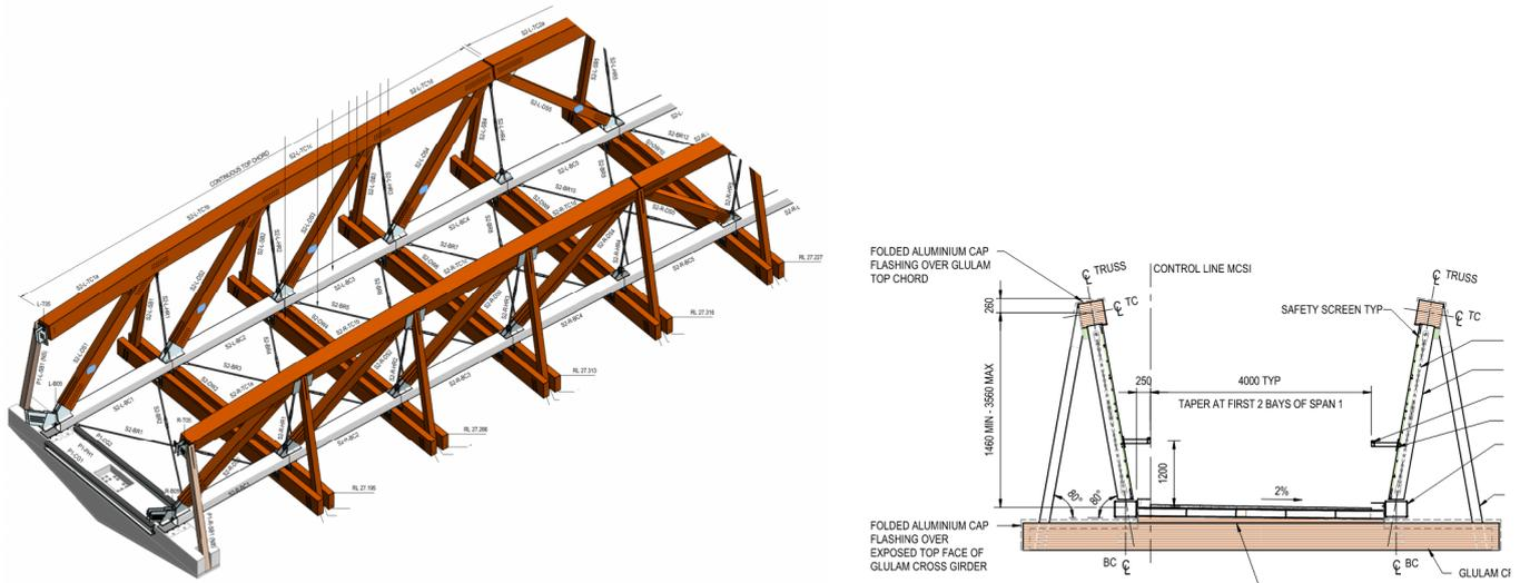
Figure 5 Half span truss isometric view and typical cross section
