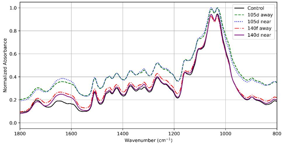
Figure 3. FT-IR spectra of wood adjacent to and 1 to 2 cm away from a galvanized connector exposed to a brown-rot fungus for 105 days (105d) and 140 days (140d)
