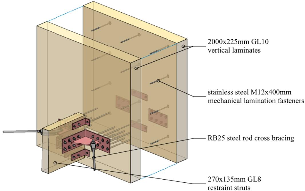
Figure 4. Exploded 3D model image of the mechanical lamination fixings
