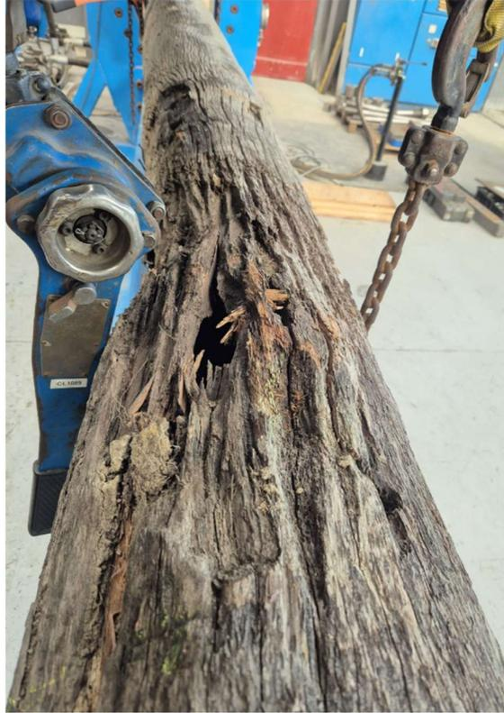
Figure 11: Pile 10 contained a void and significant degradation on the left side of the pile and buckled at the worst location, which was near the gravity support.
