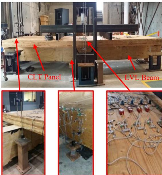
Figure 9. Experimental test set-up. (a) LVDT, (d) MTS Machine, (e) Roller Support, (f) Hinge Support, (g) Load Bearing Plate, and (h) Data Acquisition System [15].
