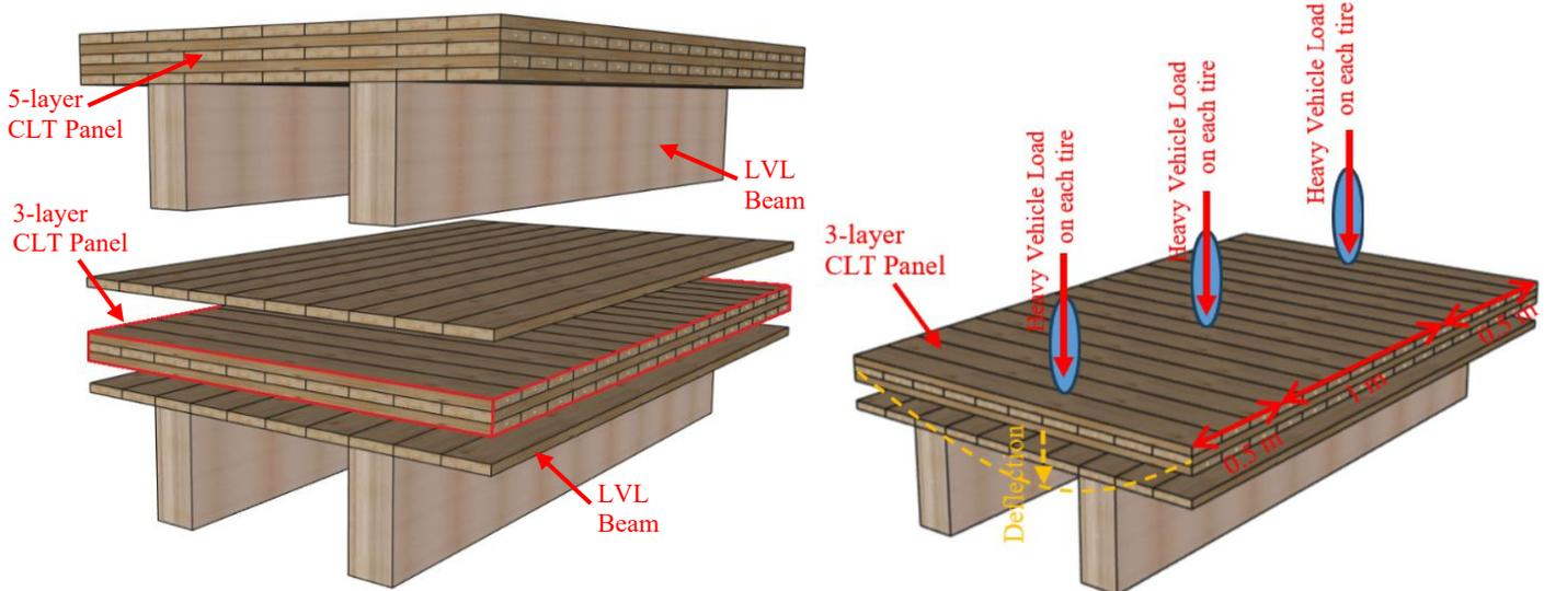
Figure 18. CLT composite double T-beam structural design concept for bridge application.
