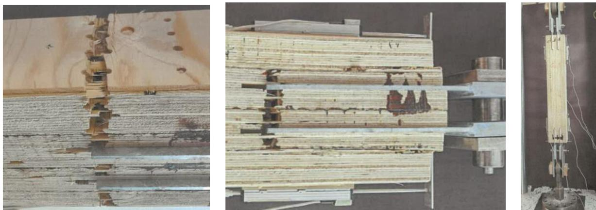
Figure 8: Tensile tests: left failure in the net section. Right failure: bloc-shear.
