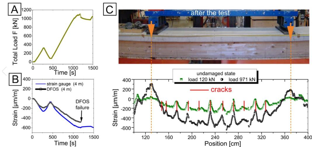
Figure 5: Load and strain data from four-point bending test of ATCC beam HBV-11; A) Load-time curve B) Strain vs. time from electrical strain gauges and DFOS in the middle of the beam (axis C) and C) Strain vs. position for loads of 120 kN and 971 kN and identified cracks (red lines) in the concrete slab
