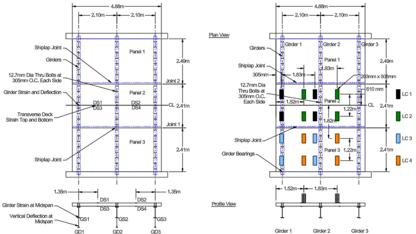
Figure 5. Three Girder Transverse Panel Configuration, Instrumentation, and Load Case Position
