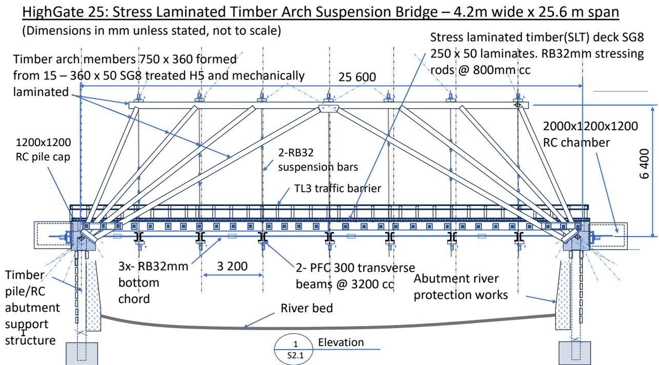
Figure 2: Concept design sketch of HighGate 25: Stress Laminated Timber Arch Suspension Bridge (25m span)
