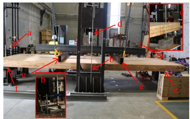
Figure 8. 500 kN MTS testing machine configured for four-point bending test. (a) LVDT 1, (d) MTS Machine, (e) Roller Support, (f) Hinge Support, (g) Load Bearing Plate, and (h) Data Acquisition System [15].
