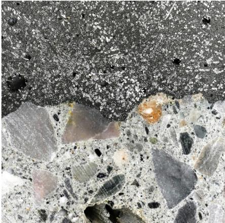
Figure 5: Comparison of UHPFRC and concrete [1]
