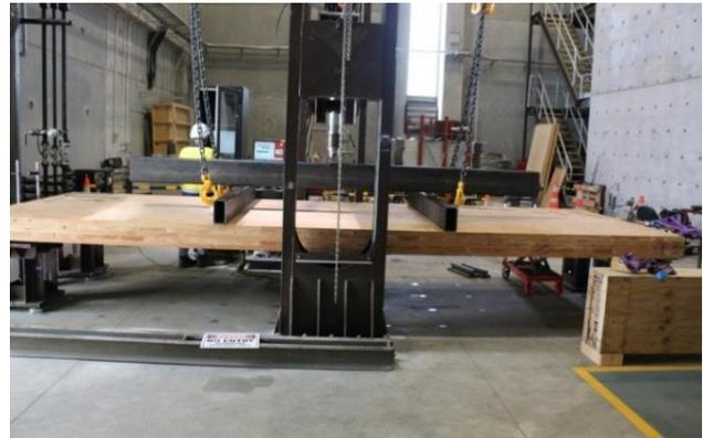
Figure 8. 500 kN MTS testing machine configured for four-point bending test [15].
