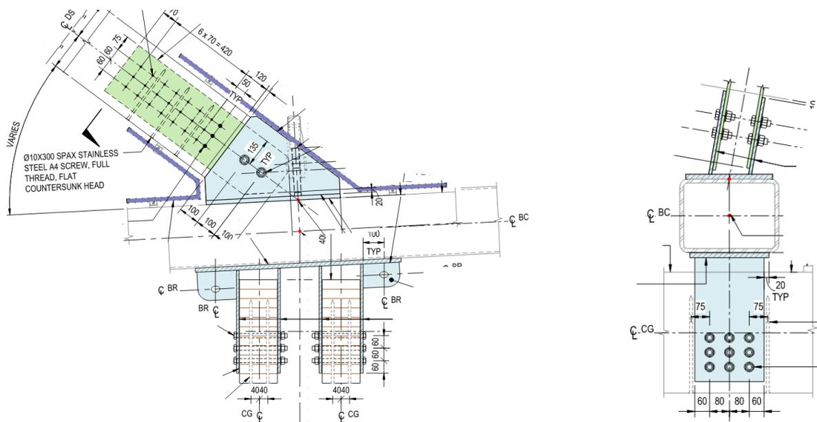
Figure 7 Typical bottom chord connection - elevation and cross section
