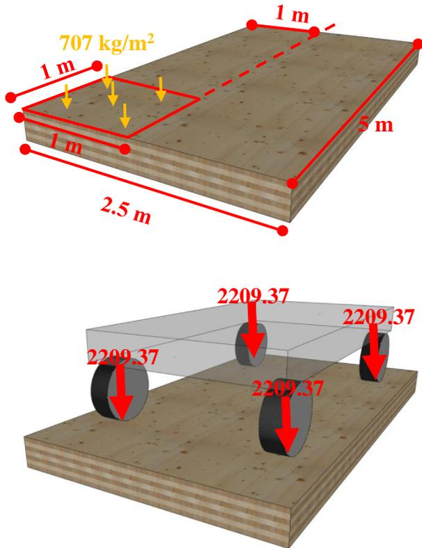
Figure 3. Uniformly loaded CLT bridge and equivalent loading for vehicle load configuration.
