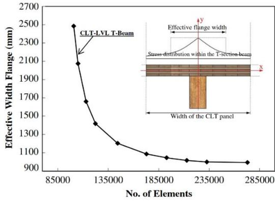
Figure 14. Convergence study result of EWF of CLT composite beam versus number of mesh elements.
