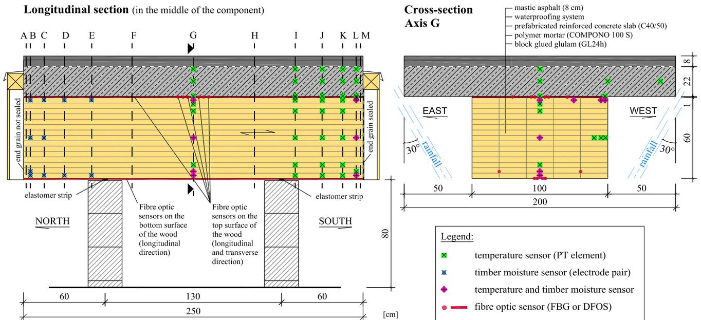
Figure 3. Superstructure segment: geometry, measuring planes and locations of the different sensors in the cross-section
