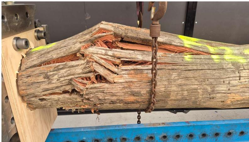
Figure 8: Compression of Pile 12 resulted in radial buckling, “mushroom”, along splits.
