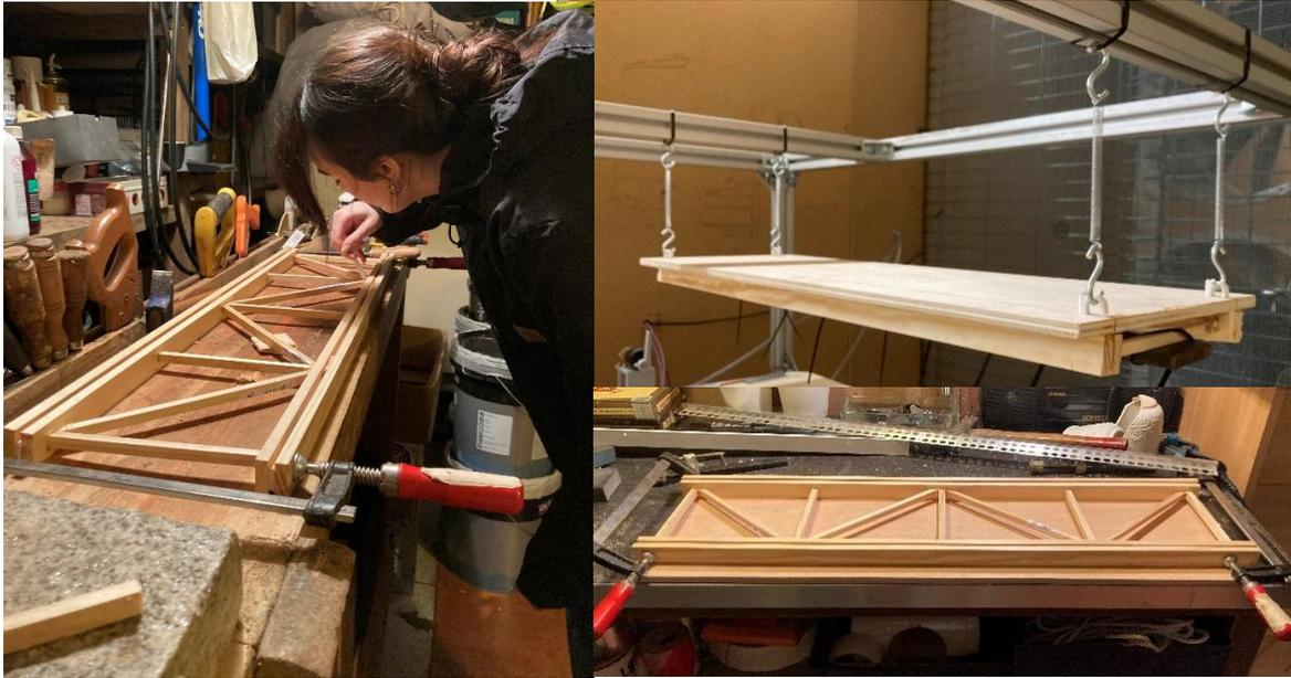
Figure 16 – Sectional model of the deck
