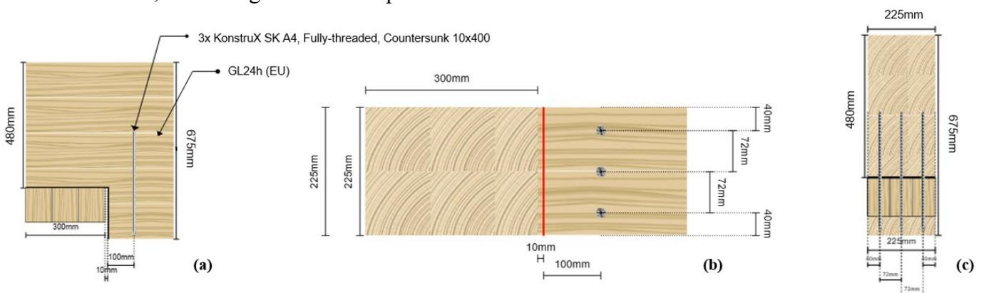
Figure 9. Reinforcement of notched beam with CLT Toolbox webtool: (a) section view, (b) bottom view, (c) side view.
