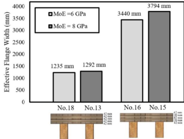
Figure 16. Effect of CLT material properties on effective flange width of CLT composite double T-beams.
