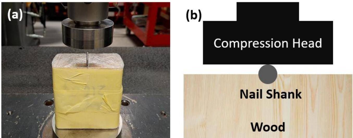
Figure 3. (a) Setup of stress relaxation tests and (b) illustration of nail shank compressed for 1.4 mm (the nail radius) into the wood block.
