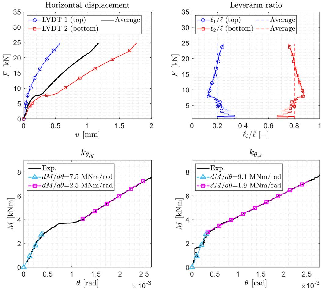
Figure 13. Top left) Horizontal displacements during the static tests of the finished arch section (see Figure 5) for bending around the y-axis. Top right) Leverarm ratios  $a_1$  (compression) and  $a_2$  (tension) for the upper and lower forces. Bottom left) Rotational stiffness around the y-axis,  $k_{\theta,y}$ . Bottom right) Rotational stiffness around the z-axis,  $k_{\theta,z}$ .
