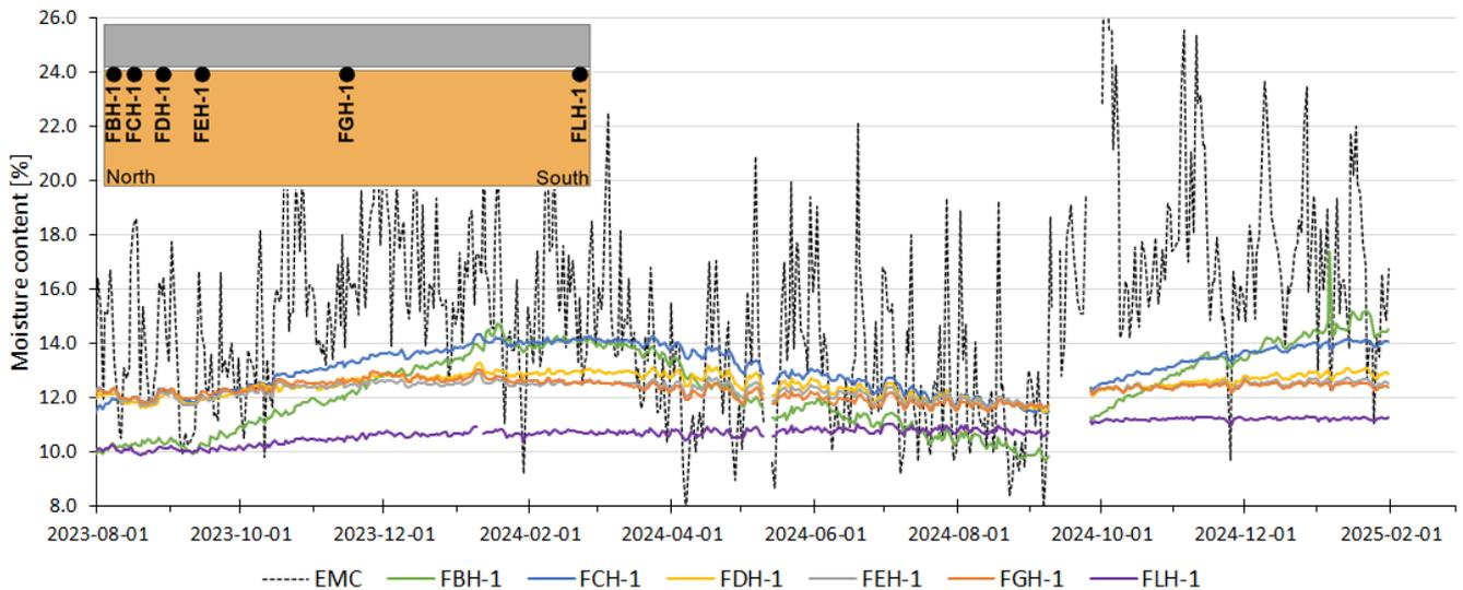
Figure 5. Daily mean values of equilibrium moisture content (EMC) and timber moisture content at several positions in the longitudinal section close to the adhesive joint
