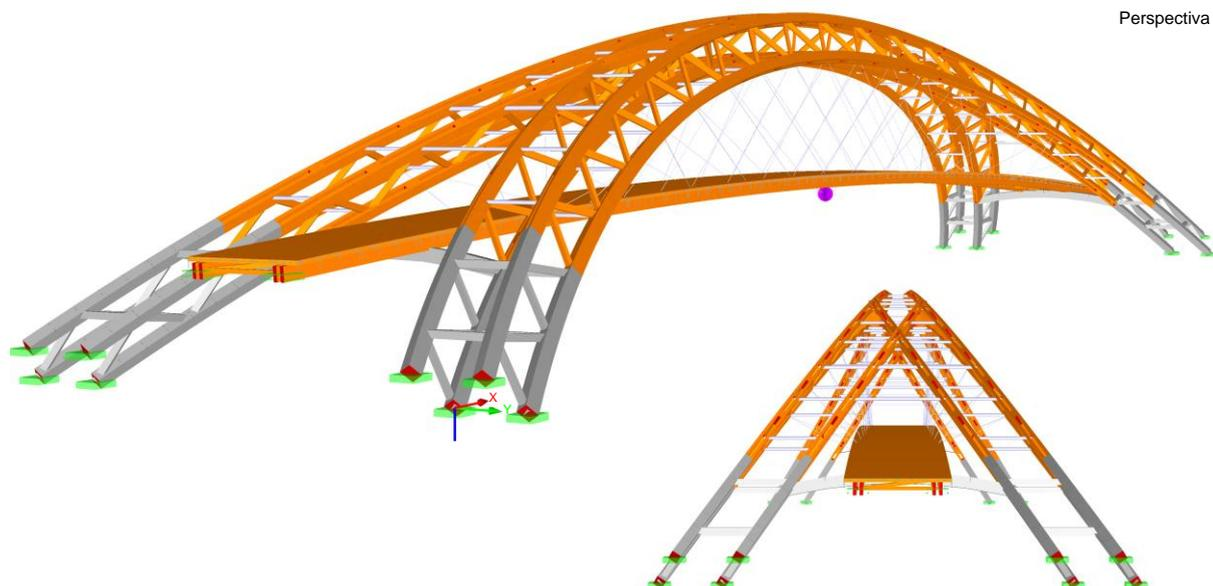
Figure 9 – Static analysis model
