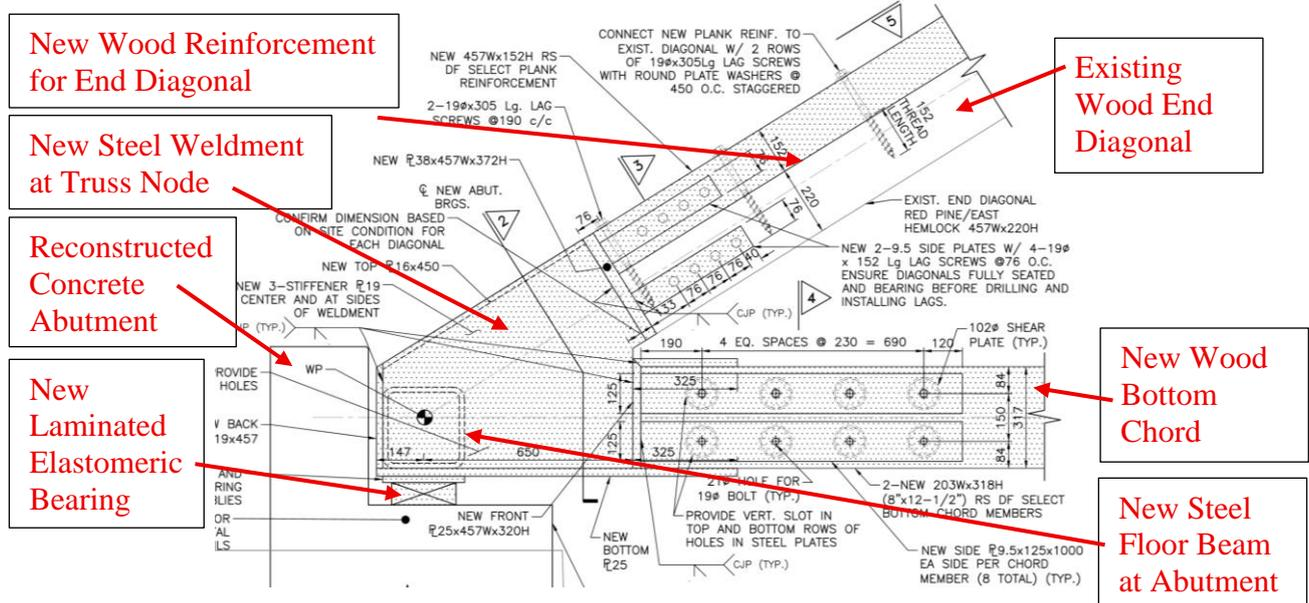
Figure 13. New wood truss end diagonal connection at bottom chord
