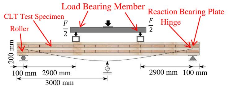
Figure 7. Test set-up for measuring the modulus of elasticity [15].
