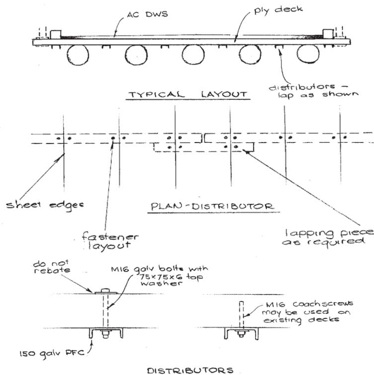
Figure 5 Indicative replacement decking layout of Drayton Rail Overbridge (Source: TMR TBMM [2])
