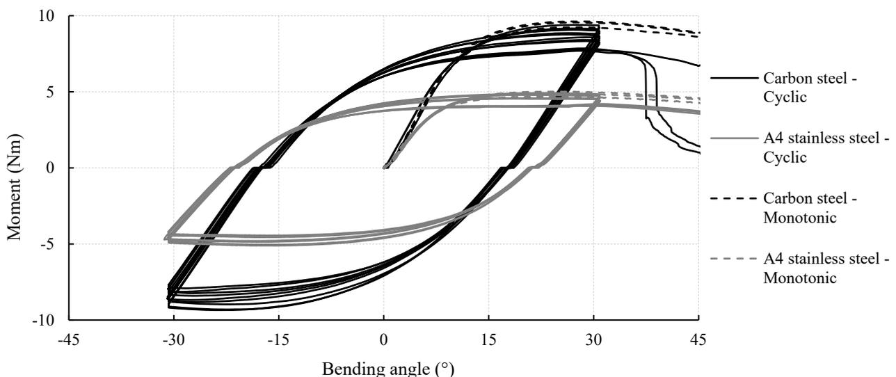
Figure 7. Cyclic bending test of partially threaded screws with nominal diameter  $d=5.0$  mm and different material, carried out by assuming a low cycle ductility class S3.
