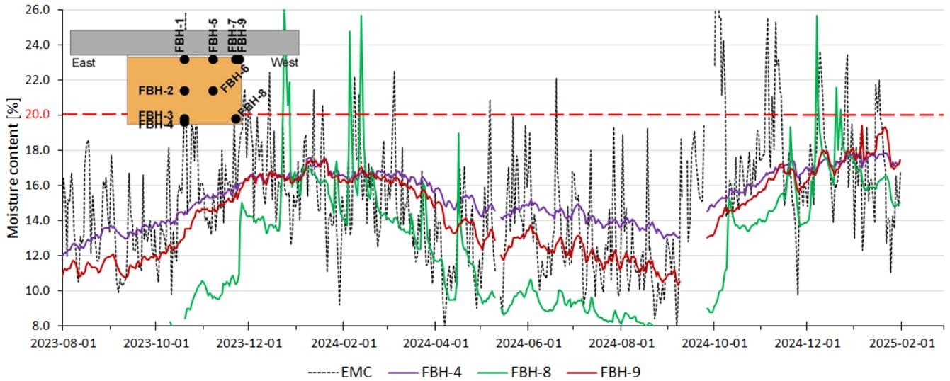
Figure 8. Daily mean values of equilibrium moisture content (EMC) and timber moisture content at three positions in measurement plane B (not sealed end grain)
