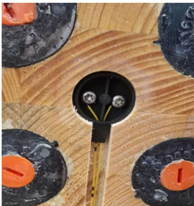
Figure 4: Resistive Sensor with protection housing
