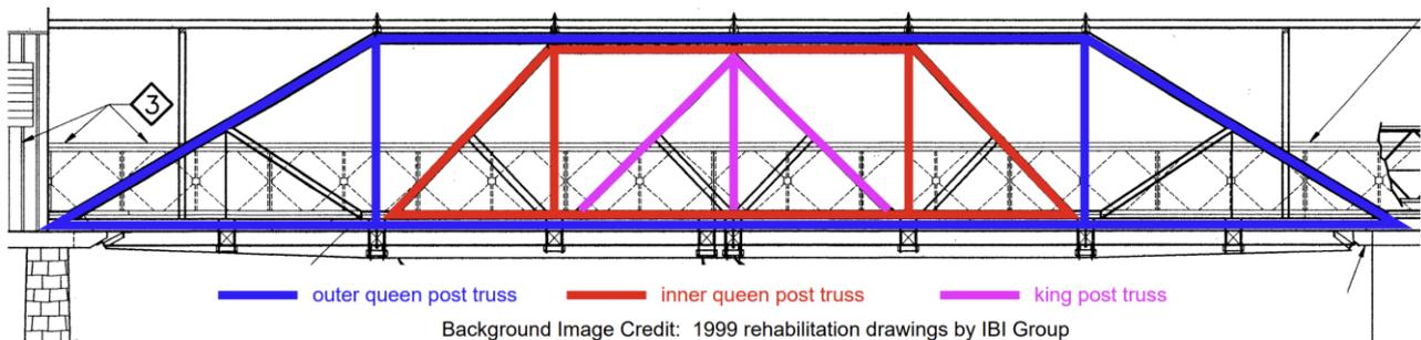
Figure 3. “Hybrid Howe” wood truss configuration of original wood trusses
