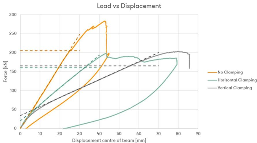
Figure 6: Results from the initial investigation of the beam clamp remedial solution.
