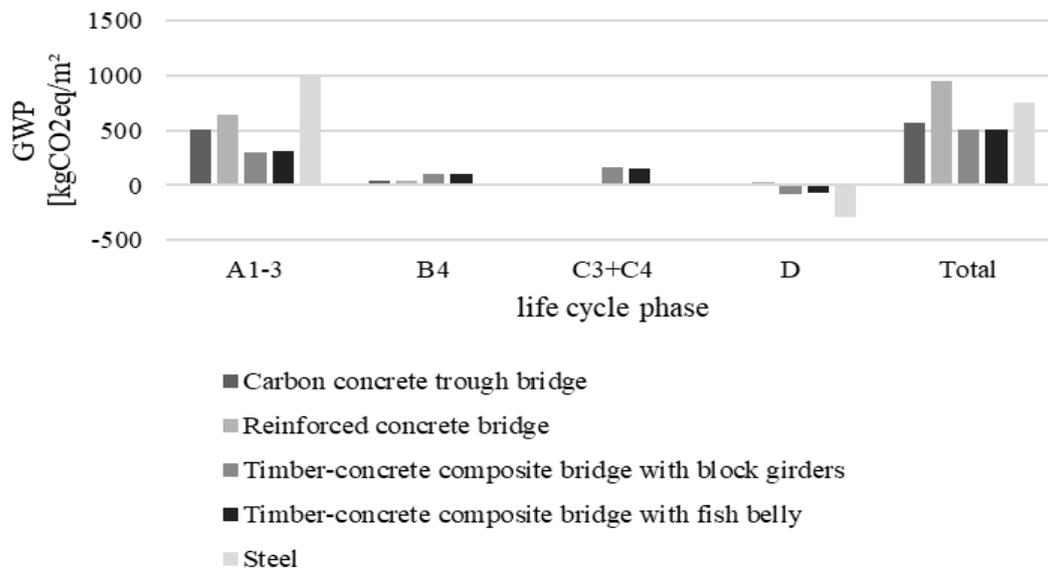
Figure 1: Comparison of the GWP results of the life cycle phases of the investigated bridge structures
