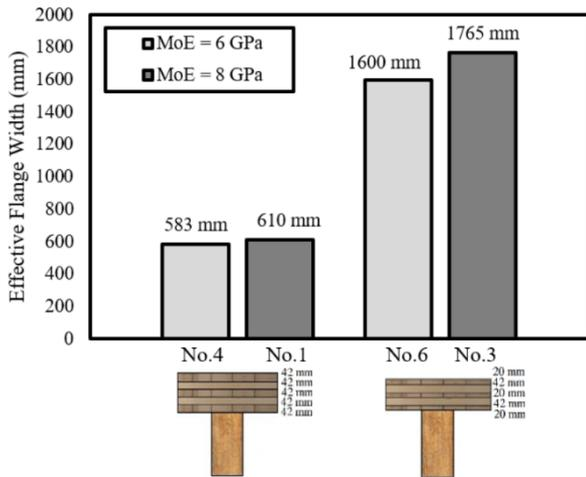
Figure 15. Effect of CLT material properties on effective flange width of CLT composite single T-beams.
