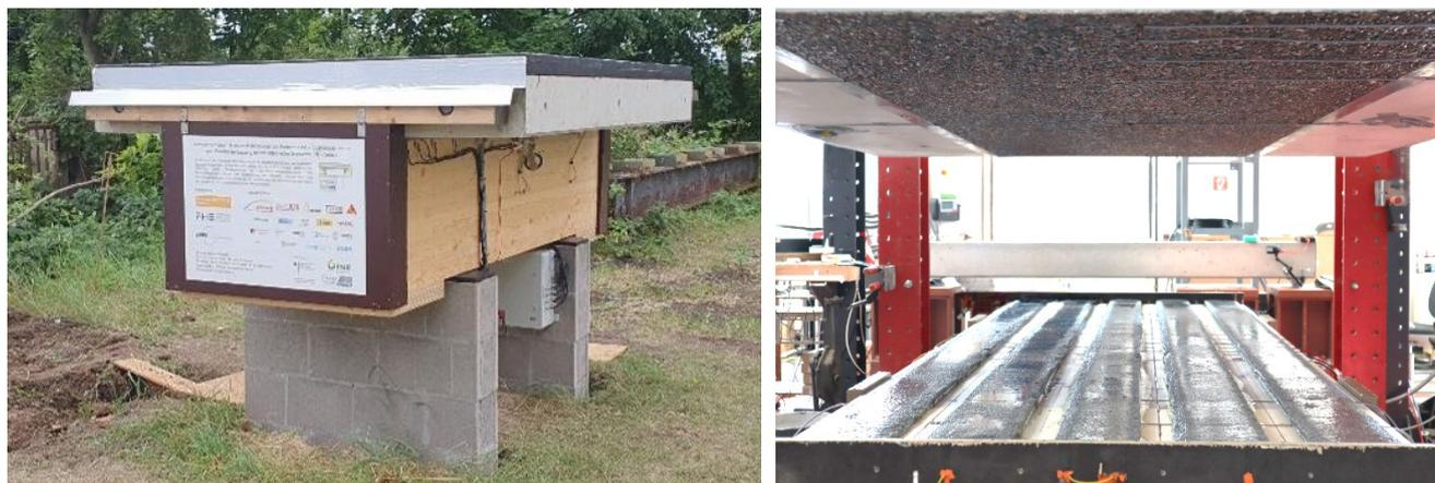
Figure 1. left: ATCC superstructure segment in outdoor climate conditions; right: Polymer mortar in strip-shape applied on the timber girder just before the concrete slab is applied from above
