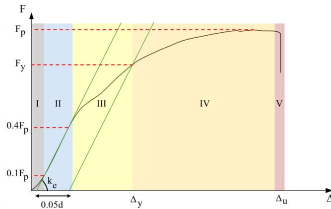
Figure 4. Typical force-displacement curve resulting from connection test containing five regions: (I) initial slip, (II) elastic region, (III) stiffness degradation, (IV) yield plateau, and (V) failure.
