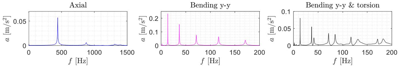
Figure 8. FFTs at stage 1 showing the resonance frequencies for free-free boundary conditions.
