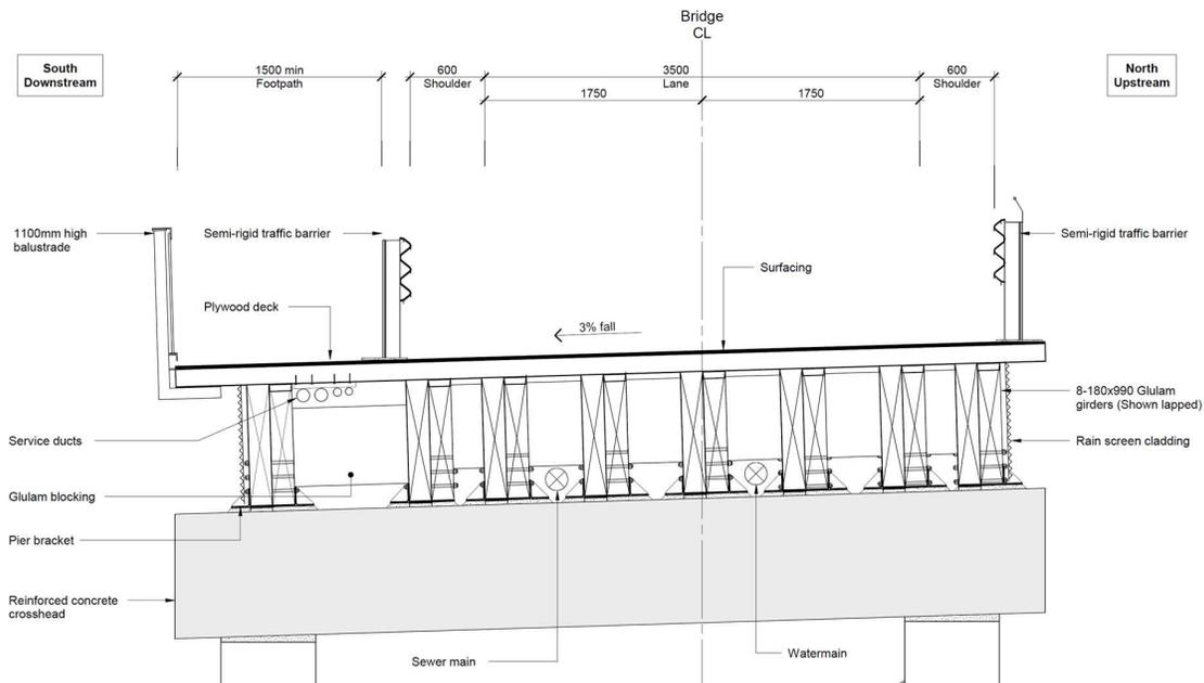
**Figure 3: Typical bridge cross section at piers.**
