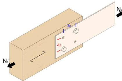
Figure 6. Connection schematic of steel plate-to-timber.
