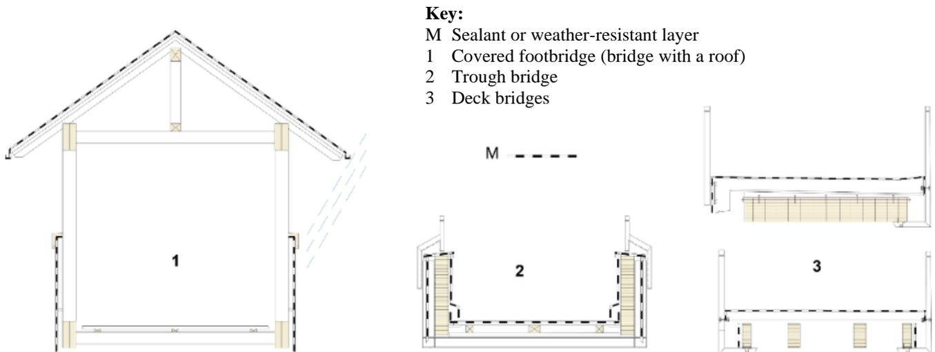
Figure 2. Examples of protected bridges (Source: FprEN 1995-2, Figure 3.2 [7])
