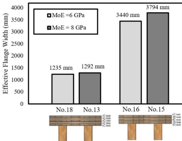
Figure 16. Effect of CLT material properties on effective flange width of CLT composite double T-beams.
