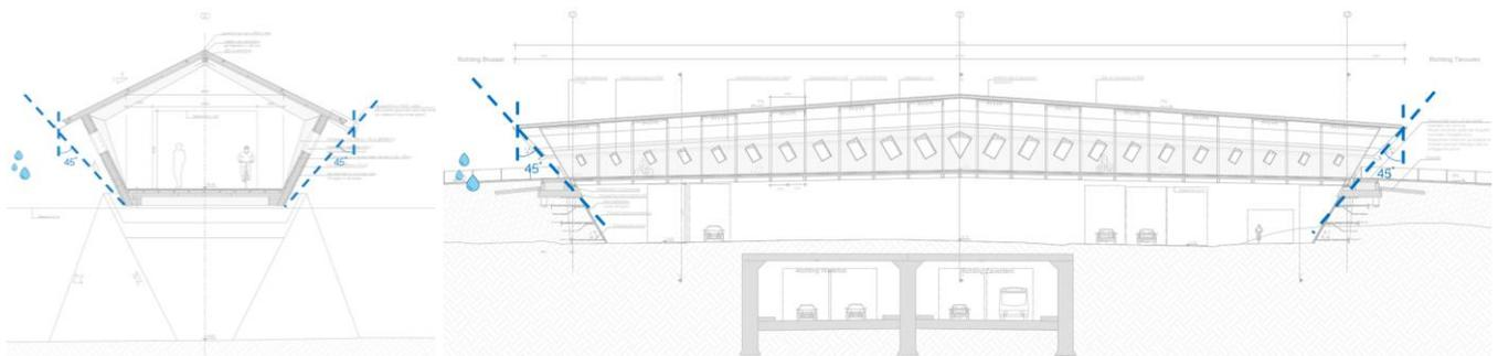
Figure 4. Geometric rules to protect timber from rain
