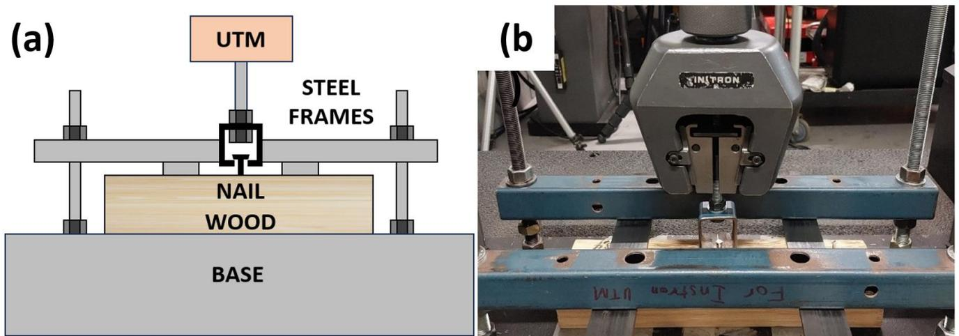
Figure 2. (a) Configuration of nail withdrawal setup and (b) a photo of the nailed assembly held by steel frames.
