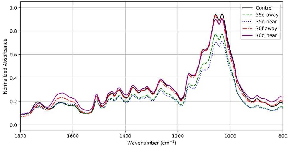
Figure 2. FT-IR spectra of wood adjacent to and 1-2 cm away from a galvanized connector exposed to a brown-rot fungus for 35 days (35d) and 70 days (70d)
