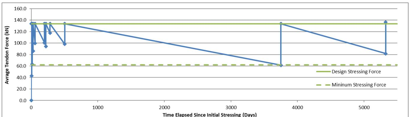
Figure 6. Loss of post-tensioning force with time over 15 years.
