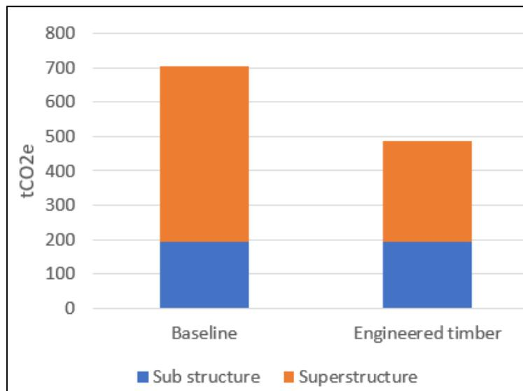
Figure 3. Graph showing carbon associated with the sub structure and super structure of a base line (Super Tee) bridge with an Engineered timber pinned arch bridge.
