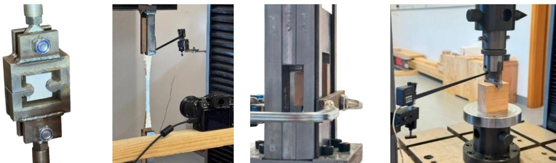
Figure 5. Mechanical tests on small clear samples from left to right: tension perpendicular to the grain, tension parallel to the grain, shear parallel to the grain, and dowel embedment test.
