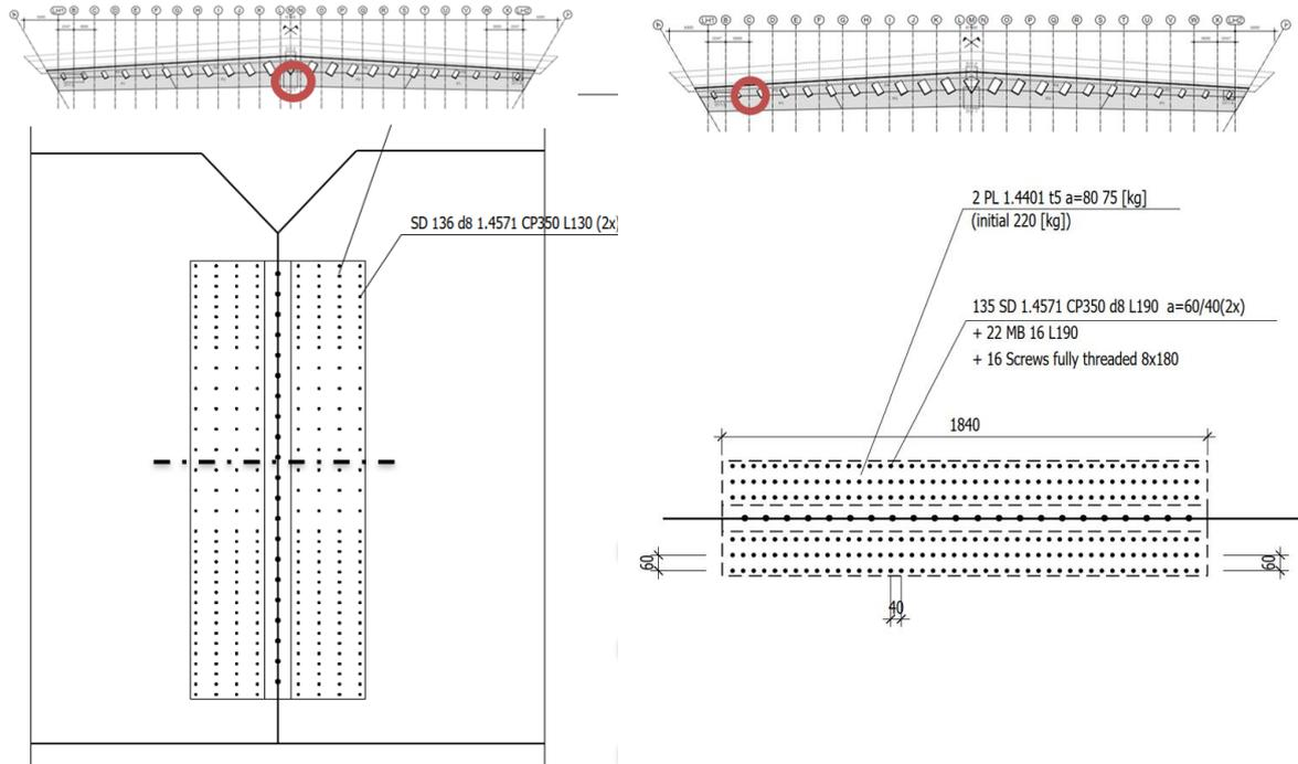
Figure 9. Connection: Left main joint in the middle of the bridge, right: Shear joint of the wall. ©sblumer
