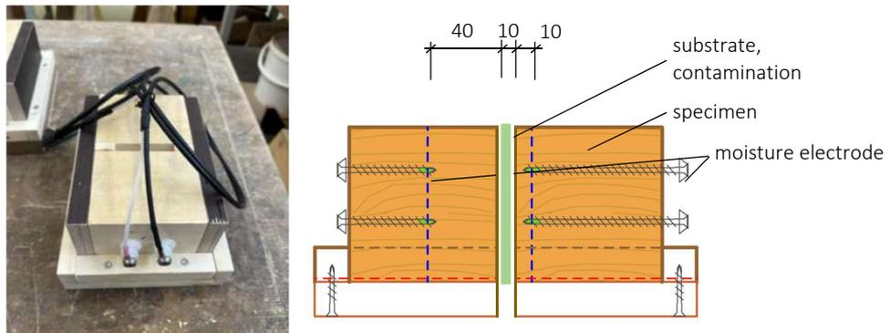
Figure 7. Test setup to measure the moisture content: two spruce wood specimens ( $435 \text{ kg/m}^3$ ) placed 10 mm apart, with a substrate in between. Moisture sensors were installed at two depths (10 mm and 40 mm) in each specimen
