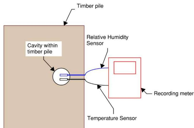
Figure 8. General arrangement of sensor installation
