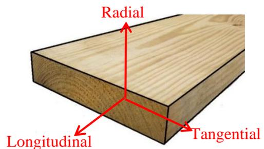
Figure 12. Principal axes of wood.
