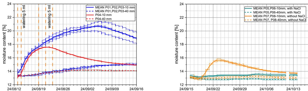
Figure 8. Influence on the moisture content of timber members, series 1 (left): wet substrate without additional NaCl, 20/65 and series 2 (right): wet substrate with/without additional NaCl, 20/65
