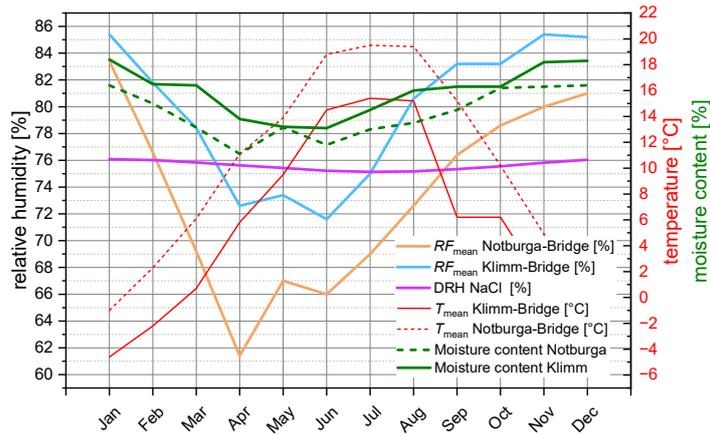
Figure 6. Climate Conditions and estimated moisture content of timber members at the locations of the Bridges
