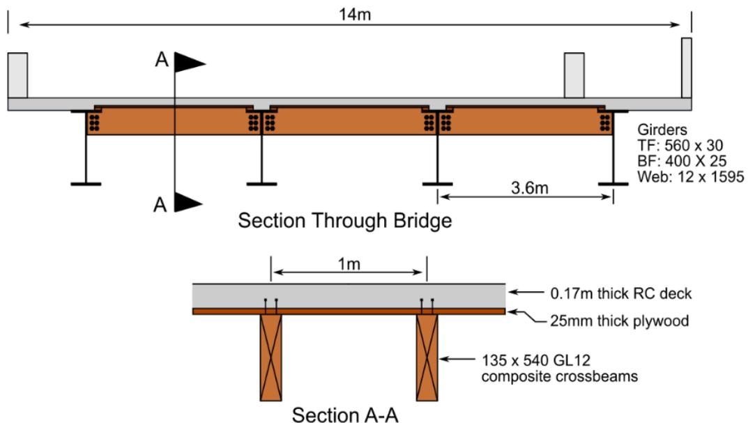
Figure 2. Proposed Composite Hybrid Bridge (CHB) Concept, showing a cross section through the bridge at midspan (top) and partial transverse section (bottom). Dimensions shown result from preliminary design.
