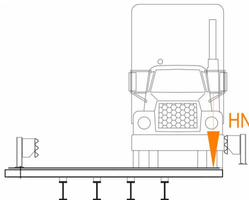
Figure 11 Sketch of load case when barrier has been knocked off
