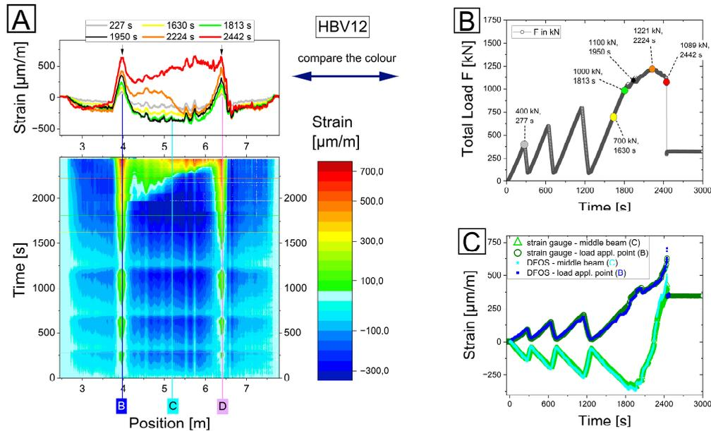
Figure 4: Fibre-optical strain data of the ATCC beam HBV-12 estimated during testing: A) Overview-plot with strain data as function of time and position; B) Load versus time plot with marked load levels for correlation to A; C) Strain-time-curves for electrical strain gauges and DFOS for load application point (axis B) and in the middle of the beam (axis C, see Figure 1)
