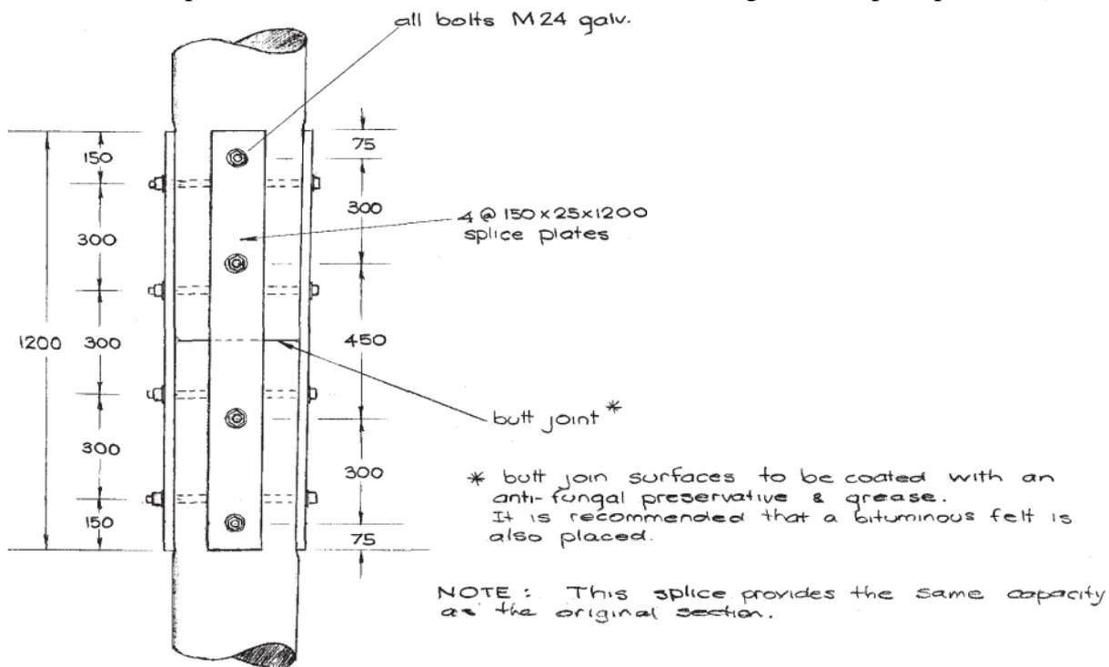
Figure 7. Pile Splice Connection Detail (Source: TMR TBMM [2])
