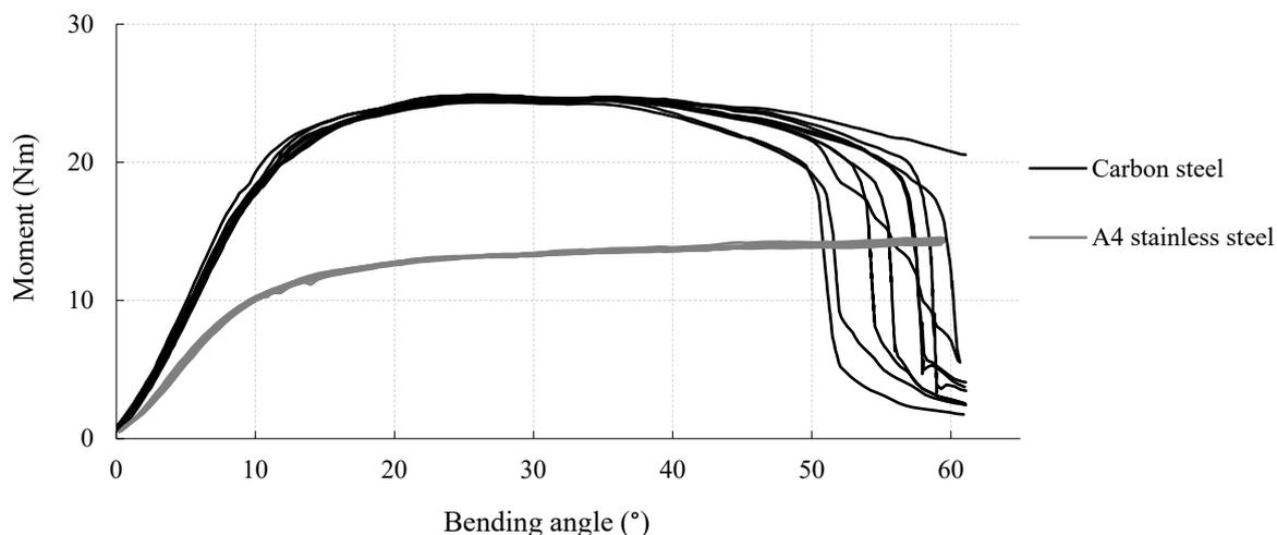
Figure 5. Monotonic bending test according to EN 409 of fully threaded screws with  $d=6.5$  mm and different material.
