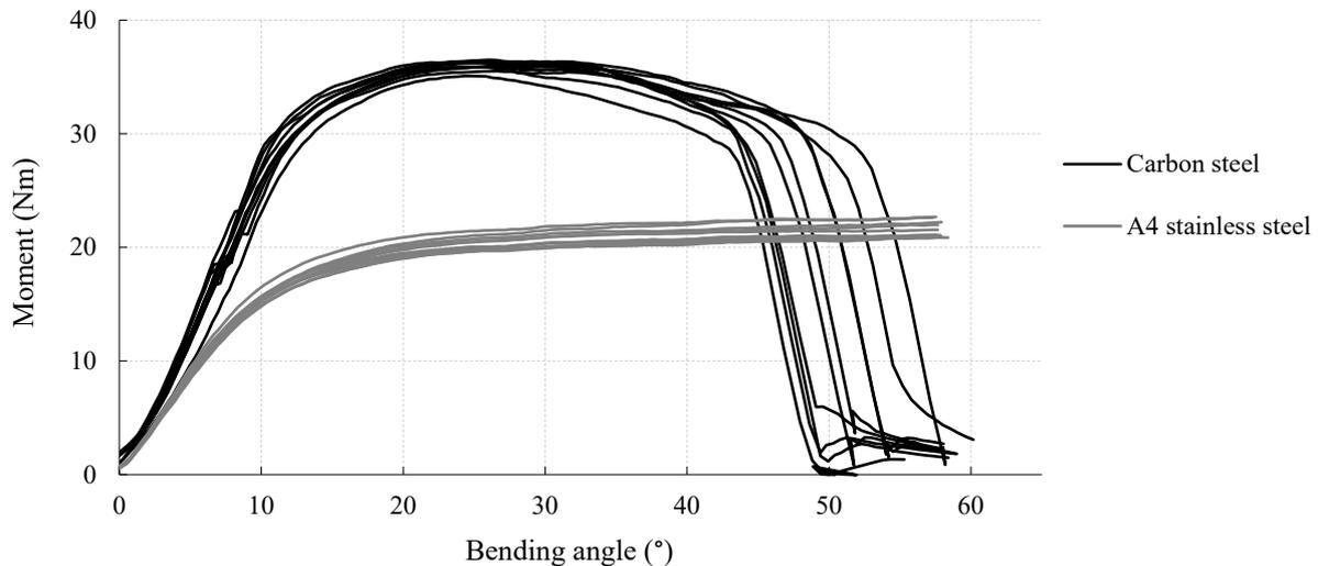
Figure 6. Monotonic bending test according to EN 409 of fully threaded screws with  $d=8.0$  mm and different material.
