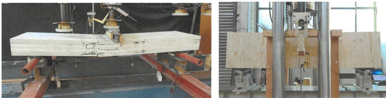
Figure 7: Three point bending tests for determination of the mechanical parameters (Left: plate, right: slab)
