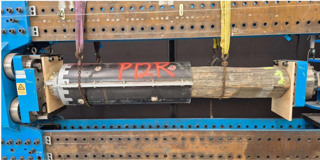
Figure 9: Pile 12 repair test setup with split cylinder and high strength grout.
