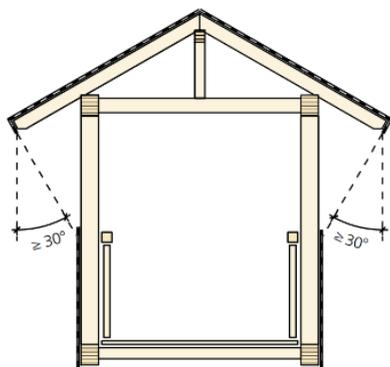
Figure 3. Covered roof bridges with gladding against driving rain, source: [9]
