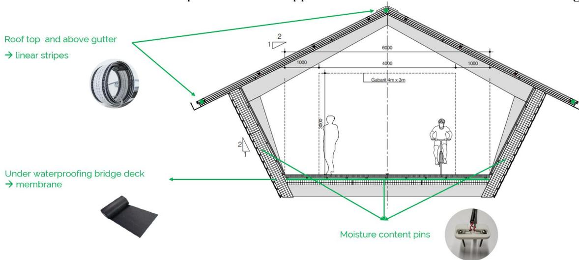
Figure 5. Implementation of monitoring system
