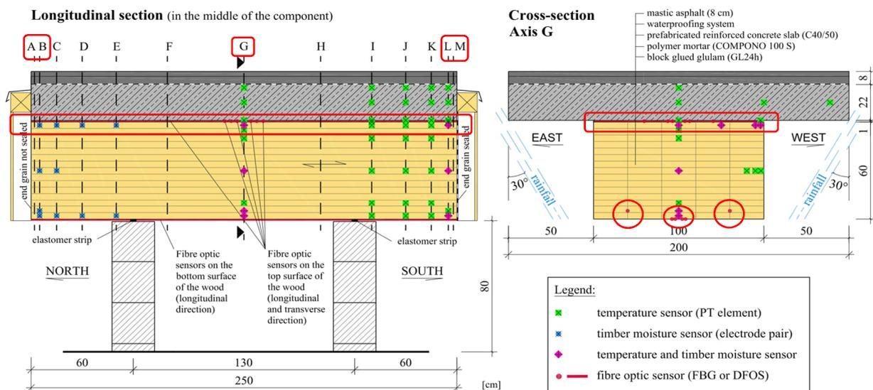
Figure 2: Superstructure segment the sensor positions (A to M). (The positions of the fibre-optical sensors are marked in red.)
