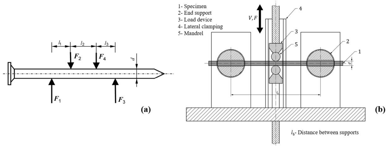
Figure 4. Bending tests of dowel-type fasteners: (a) free body diagram of monotonic test according to EN 409 [13], (b) setup of cyclic loading test according to EN 14592 [10].
