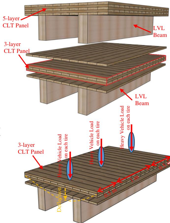
Figure 18. CLT composite double T-beam structural design concept for bridge application.
