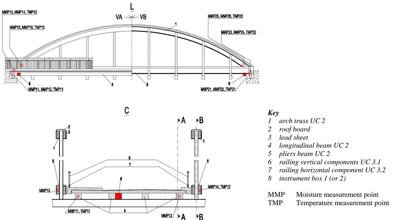
Figure 5. Moisture monitoring – example arch truss (Source: FprEN 1995-2, Figure D.13 [7])
