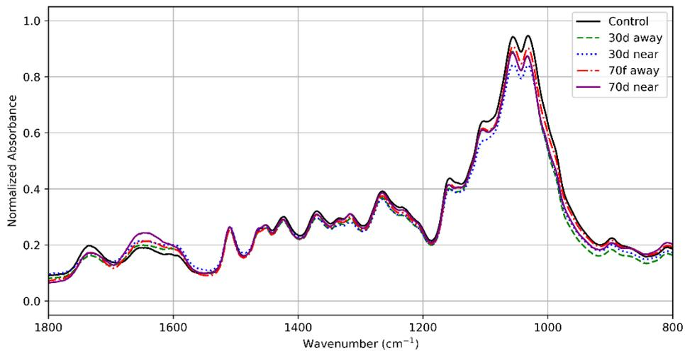
Figure 4. FT-IR spectra of wood adjacent to or 1 to 2 cm away from a stainless steel connector exposed to a brown-rot fungus for 35 days (35d) and 70 days (70d)
