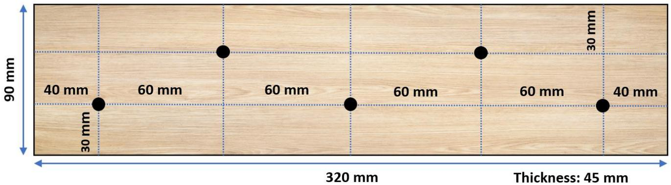
Figure 1. Configuration of a nailed assembly for nail withdrawal tests. Black dots represent the driving positions of nails.
