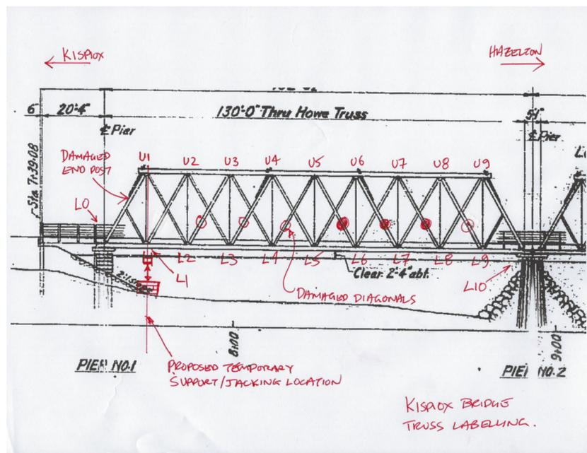
Figure 10. Sketch Showing Damaged Diagonals and Temporary Shoring Point
