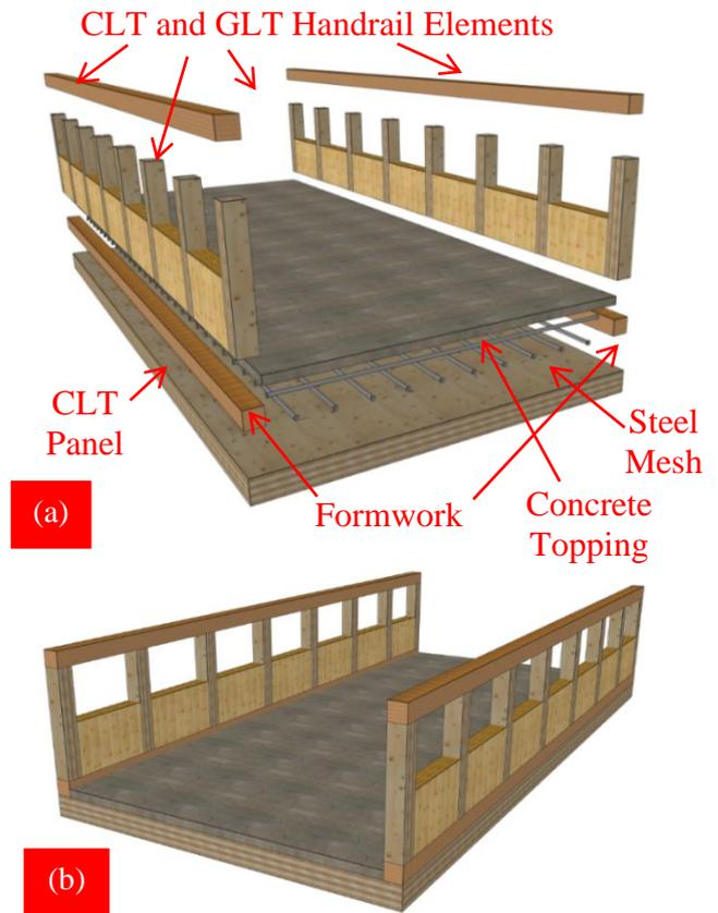
Figure 4. Prefabricated CLT bridge; a) before assembly, b) after assembly.
