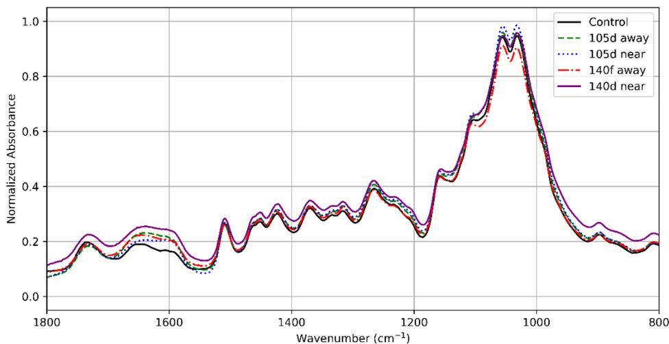
Figure 5. FT-IR spectra of wood adjacent to or 1 to 2 cm away from a stainless steel connector exposed to a brown-rot fungus for 105 days (105d) and 140 days (140d)
