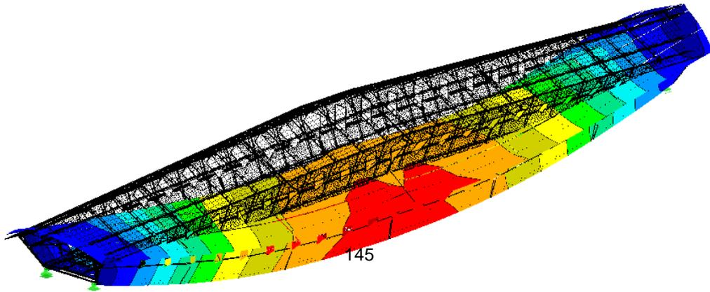
Figure 11. Vertical deformation of the bridge under self-weight (less than 5% variation to measurement) ©sblumer
