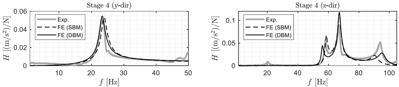
Figure 12. FRFs at stage 4 from hammer excitation and acceleration in the y- and z-direction.
