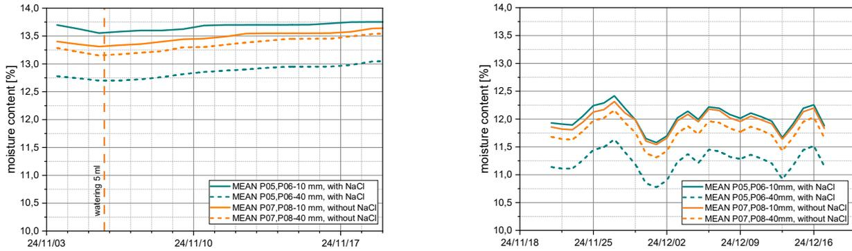
Figure 9: Influence on the moisture content of timber members, series 3 (left): dry substrate with/without NaCl and series 4 (right), 20/85: dry substrate with/without additional NaCl, variabel
