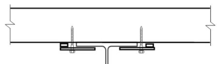
Figure 8 Sketch of coach bolts clamping EPP to top flange
