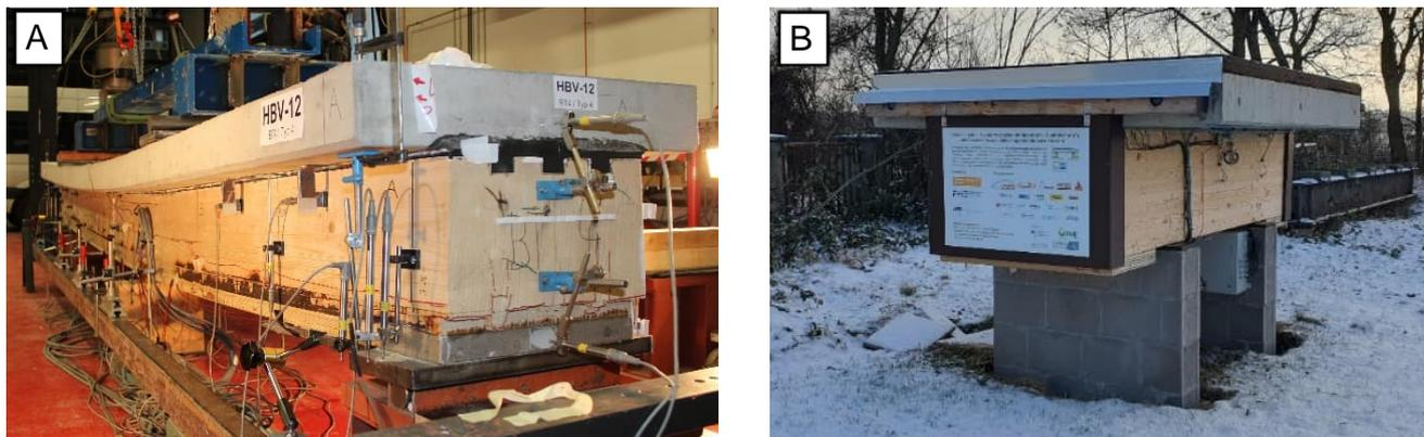
Figure 3: A) ATCC beam HBV-12 under bending load and B) ATCC-superstructure segment in outdoor climate in Weimar, Germany (January 2024)
