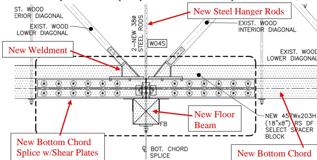
Figure 12. Typical rehabilitated wood truss details at bottom chord splice
