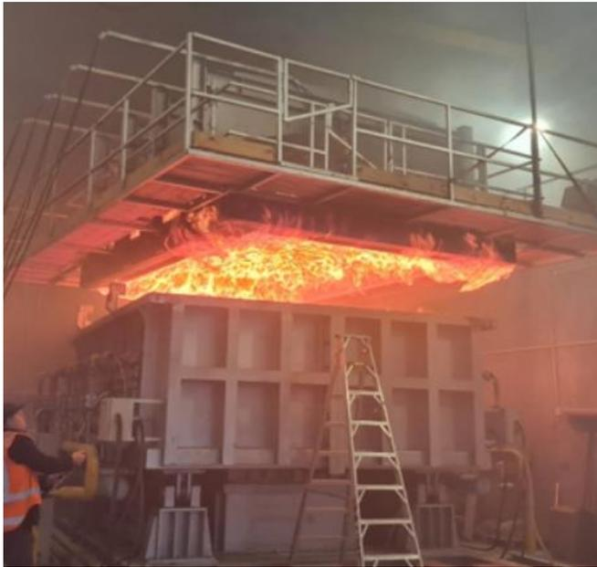
Figure 6. Red Stag CLT fire test.
