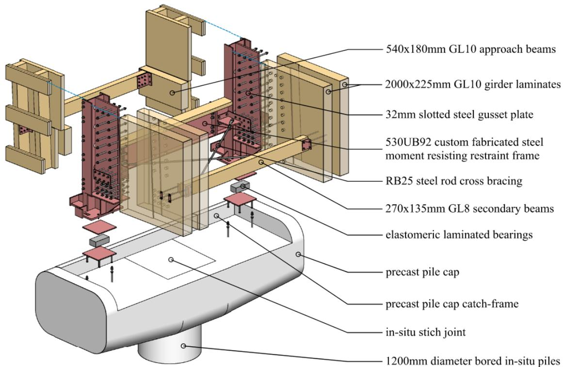
Figure 2. Exploded 3D model image of the superstructure at the end of the bridge main span
