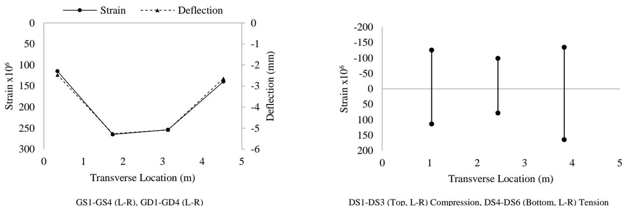
Figure 7. Girder Strain and Deflection (left) and Transverse CLT Panel Strain (right) - Four Girder Assembly
