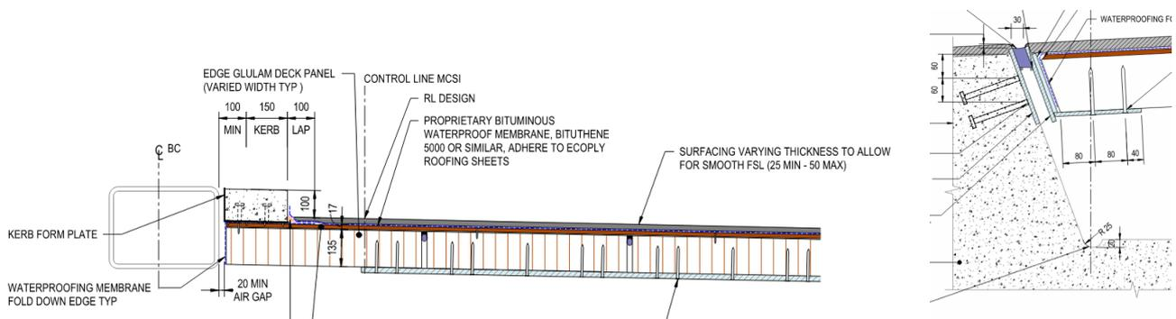
Figure 8 Glulam deck plate – typical cross section and expansion joint detail
