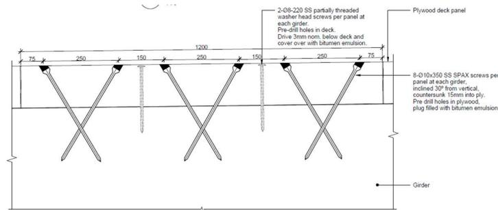
Figure 6: Plywood deck panel to girder connection detail
