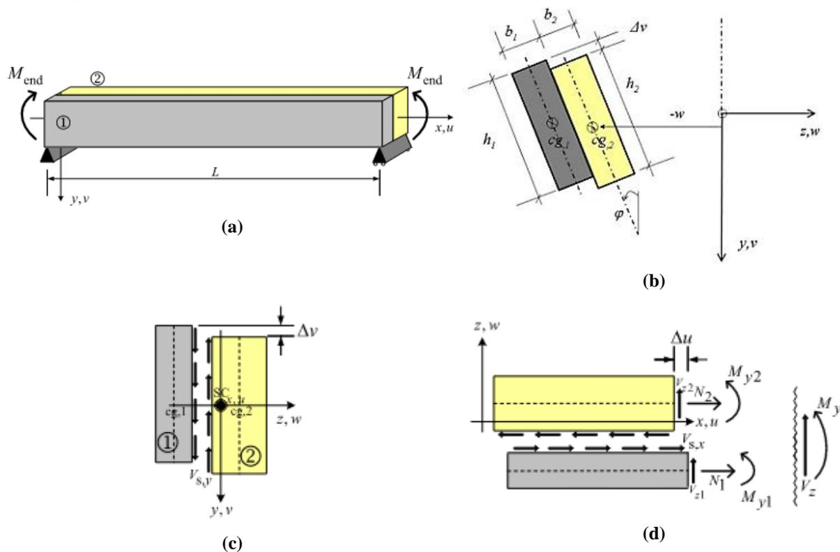
**Figure 3.** (a) Beam member boundary conditions for analytical model. (b) Simplified kinematics of a partially vertically layered composite section. (c) Cross section view of beam with slip forces in the cross-longitudinal or vertical direction. (d) Vertical view of beam element with transverse forces and moments defined positive as shown, including slip forces in the longitudinal or horizontal direction [3]
