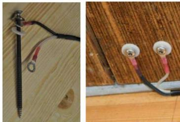
Figure 7. Chrome-steel electrodes installed into timber members [26]
