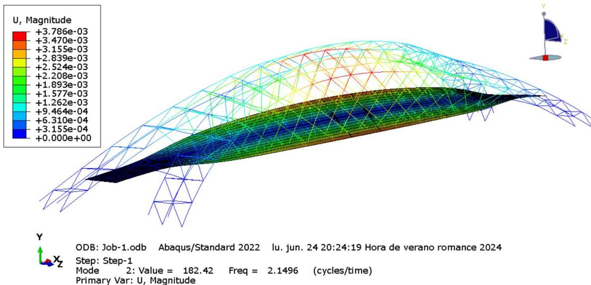
Figure 11 – Natural frequency with the highest likelihood of resonance
