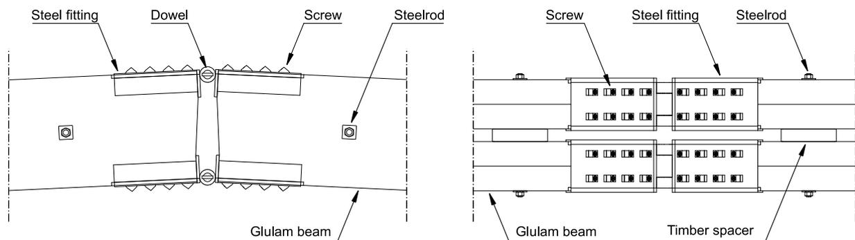
Figure 2. Steel hinge connection.
