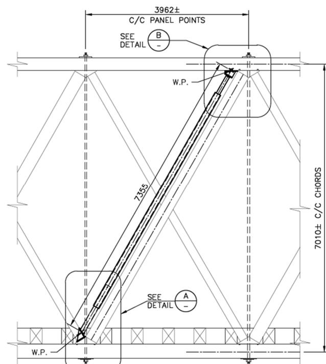
Figure 12. General View of Deployed Jacking Strut
