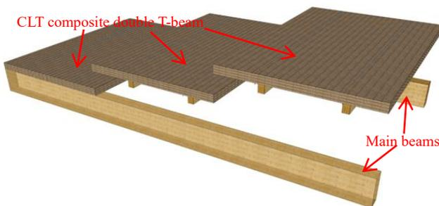
Figure 17. Intermediate Span CLT composite double T-beams.
