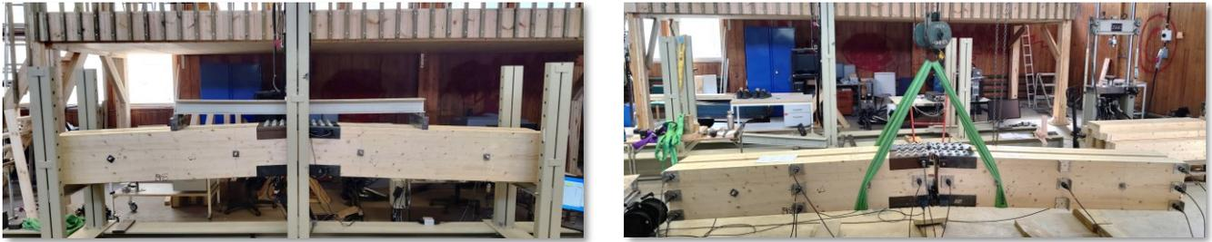
Figure 3. Left) Static four-point loading. Right) Dynamic testing with free-free boundary conditions.
