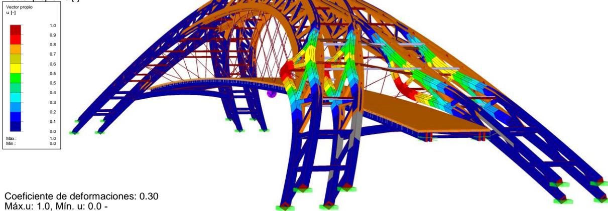
Figure 10 – Buckling calculation
