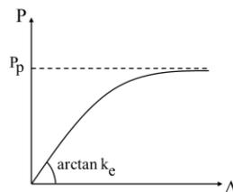
Figure 1. Mechanical model of the embedded bolt in wood [9].
