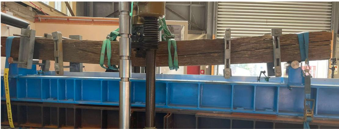
Figure 5: A beam specimen with horizontal restraint clamps.
