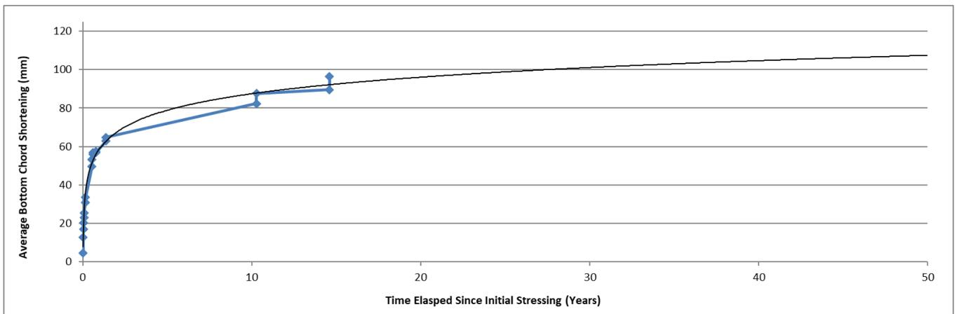
Figure 9. Predicted compressive distortion of the bottom chord over 50 years.
