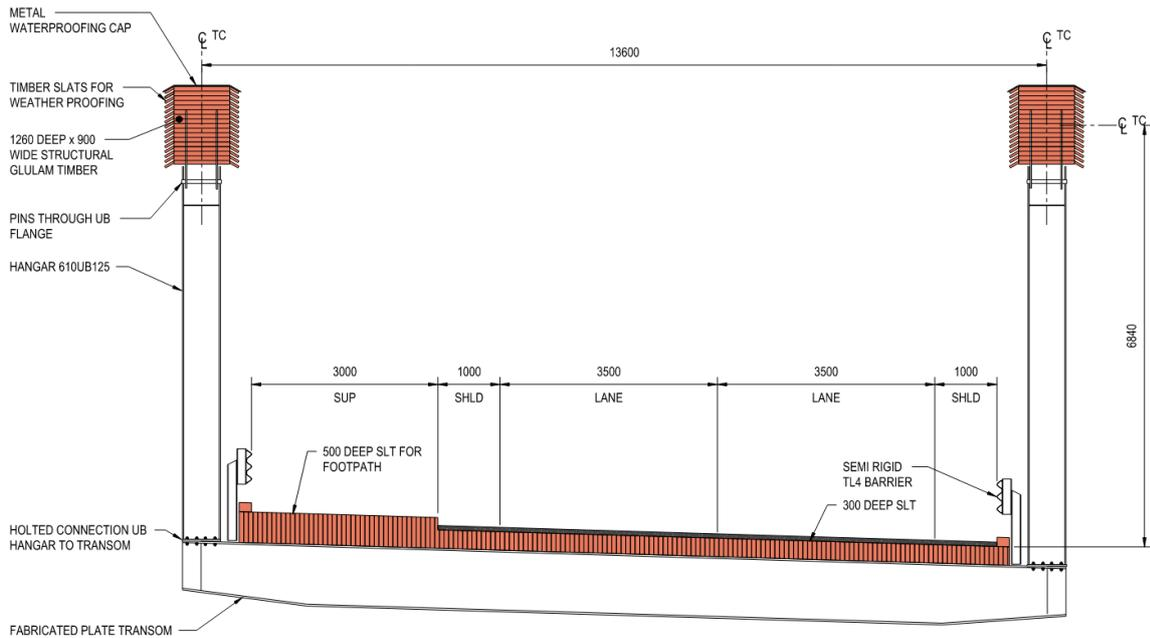
**Figure 2 Concept general arrangement cross section.**
