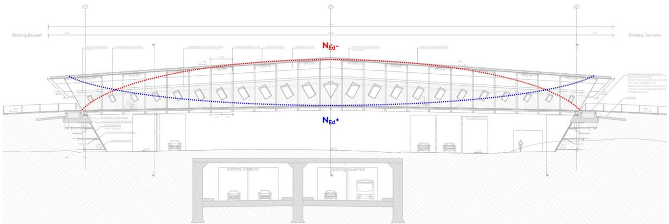
Figure 6. Flow of forces in the timber box girder
