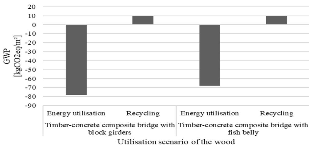
Figure 2: Recycling Potential Assessment of the two investigated timber bridge constructions
