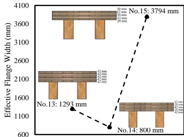
Figure 14. Effect of the layer's configuration change on the effective flange width for Configurations 13, 14, 15.
