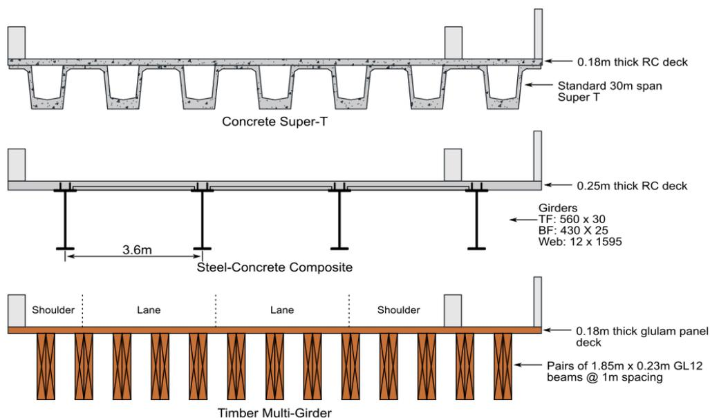
**Figure 3: Cross section of conventional construction materials bridge configurations with dimensions from preliminary design.**
