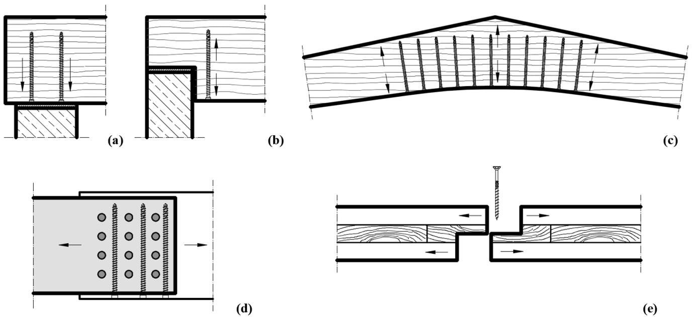
Figure 2. Application examples of modern wood screws: (a) compression reinforcement of support areas, (b) tension reinforcement of notched beams, (c) apex tension reinforcement of pitch cambered beams, (d) reinforcement of dowel-type connections, (e) half-lap joint of CLT panel
