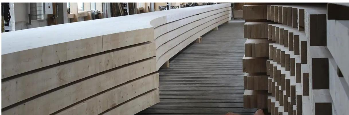
Figure 3 Single elements before block lamination by Schaffitzel
