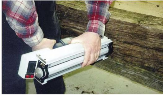
Figure 6. Resistance drilling method has been used for assessing timber internal condition [23]
