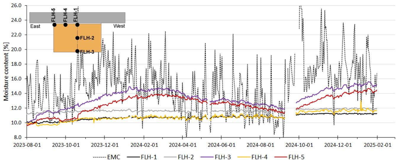
Figure 6. Daily mean values of equilibrium moisture content (EMC) and timber moisture content at several positions in measurement plane L (sealed end grain)
