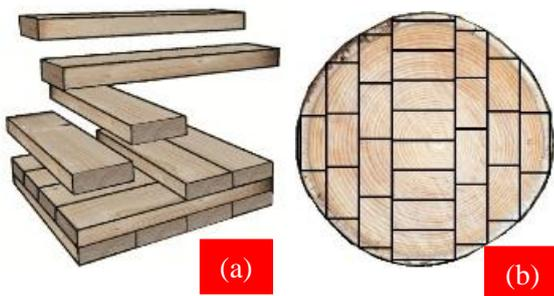
Figure 1. CLT production process; (a) Sawing log, (b) Arranging boards and final CLT product.
