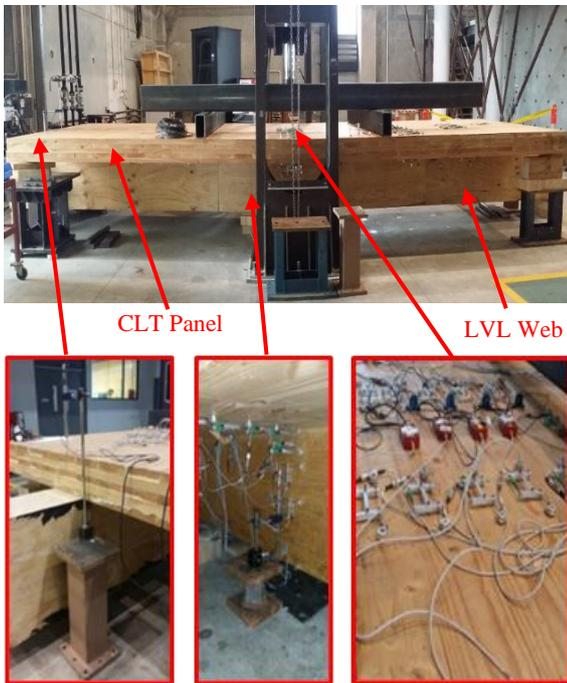
Figure 9. Experimental test set-up. (a) LVDT, (d) MTS Machine, (e) Roller Support, (f) Hinge Support, (g) Load Bearing Plate, and (h) Data Acquisition System [15].
