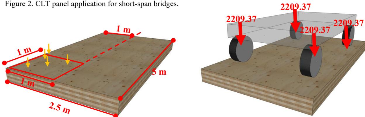
Figure 3. Uniformly loaded CLT bridge and equivalent loading for vehicle load configuration.
