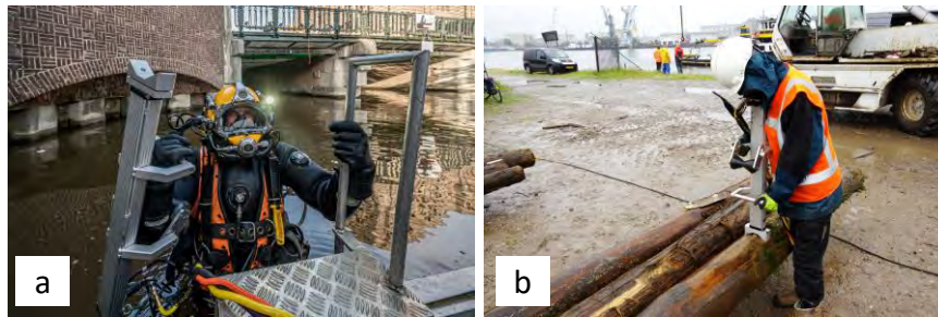
Figure 4: Micro-drilling measurements: a) underwater measurements on wooden piles; b) measurements after piles extraction.
