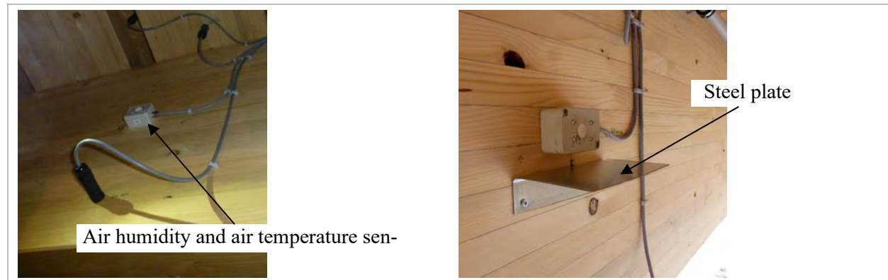
Figure 4 Air humidity and air temperature sensor (left) and steel plate as radiation protection (right).
