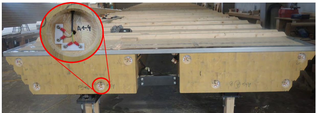
Figure 6: Cross-sectional end grain face view of the superstructure GLT block girders with 2x4 measuring points, each with 2 pairs of electrodes for moisture measurement
