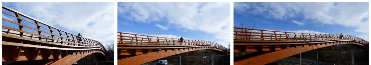
Fig. 9. Transits on the footbridge. A single pedestrian walking test.
