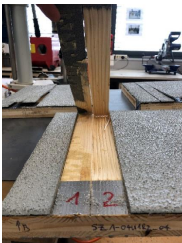
Pic.3: Peel test, System 1
