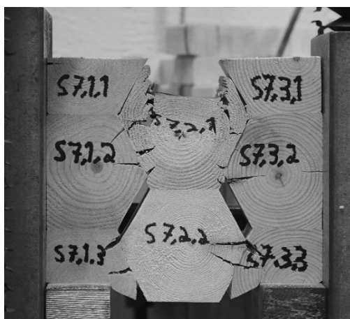
Figure 6: Shear test failure of oblique interlocked lamellae [2]
