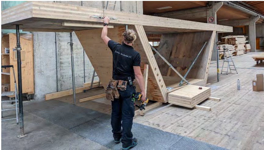
Figure 18: Manufacturing box-girder modules at the factory. Picture: Flück AG, Wangen b. Dübendorf
