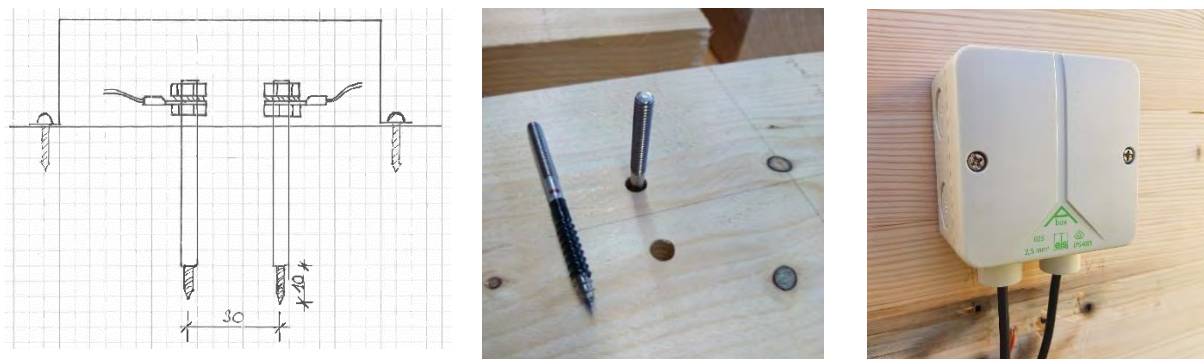
Figure 3: Principle sketch and photos of the installation of the hanger bolt electrodes and protective box, [11]
