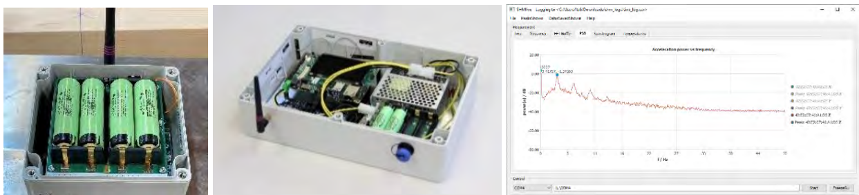
Figure 16: Sensor node with 3-axis acceleration sensor below the battery pack (left), HUB (center) and FFT analyses of the frequencies (right)
